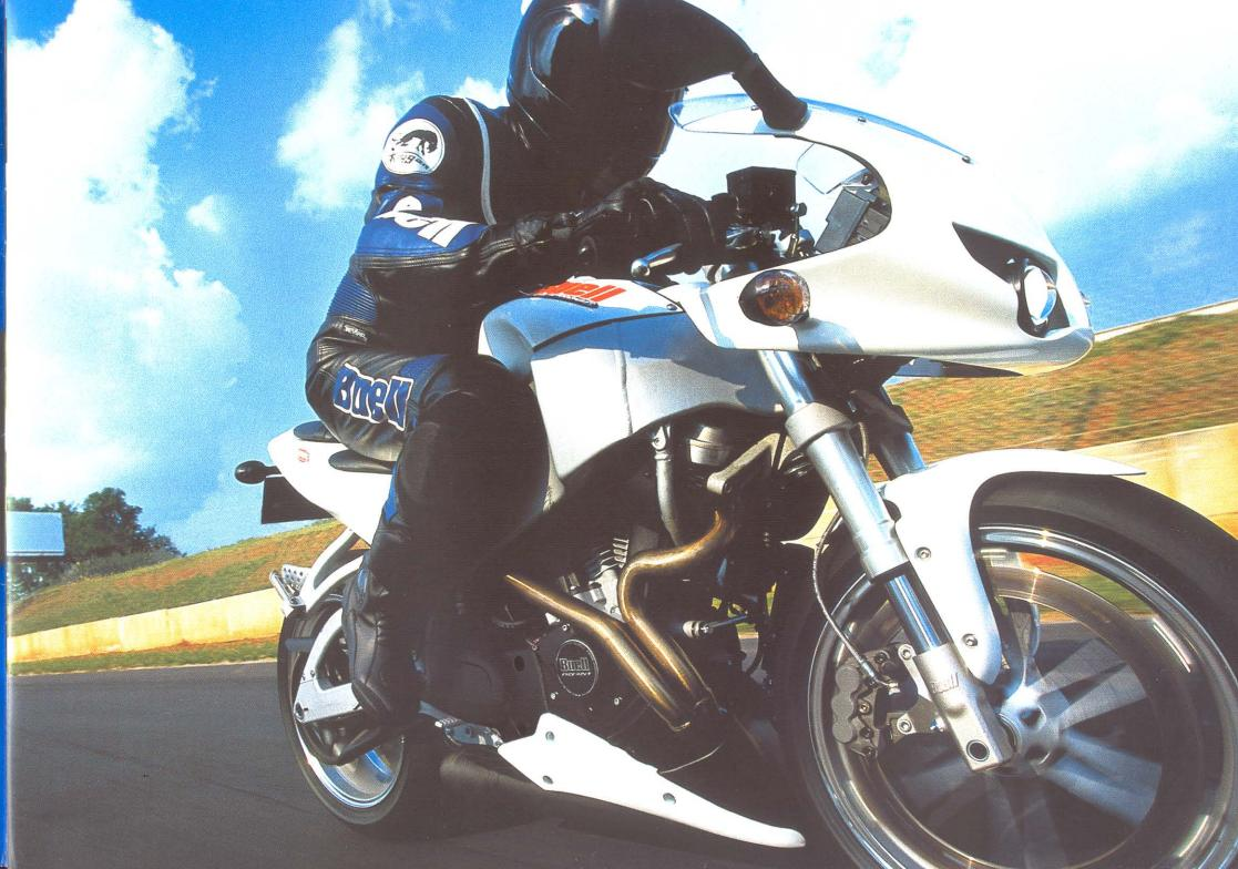
To get an idea of where the Firebolt is coming from, we need to examine its heart – a pushrod, fuel-injected, forced air-cooled, 45 degree V-twin. It's all new – from the crankcases up – and its 984 cubic 'C's punch out a controllable 92bhp, delivered via smooth and low-maintenance belt-drive.
