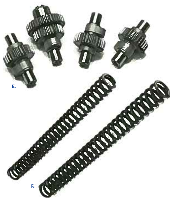
F. Lightning Series Race Fork Spring Set Used by the Lightning Series race teams in the States, stronger fork springs reduce front end dive under hard braking conditions. #45989-96Y Fits: Lightning '96-'98, White Lightning '98, Thunderbolt '97-'98.
