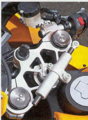
ABOVE Bar-mounted steering damper is unadjustable
