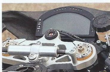
The dash, the damper, the Öhlins. The Buell is littered with desirables.
