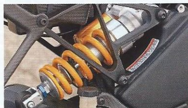
The offset TTX36 Öhlins rear shock gives a clue as to the refined handling you can expect from this beauty.
