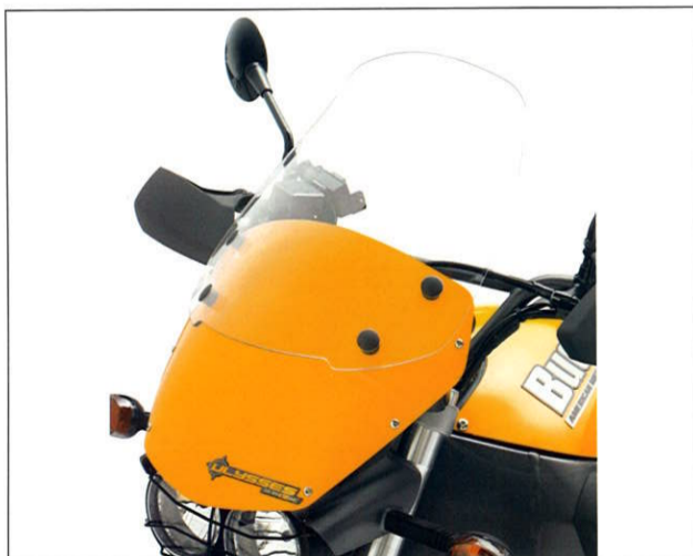
Quick-release two-piece tall windscreen means effective air flow.
