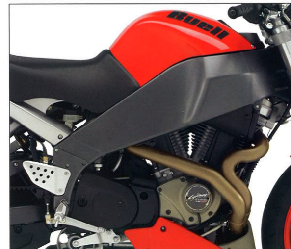
Larger frame increases fuel capacity to 4.4 gallons.
