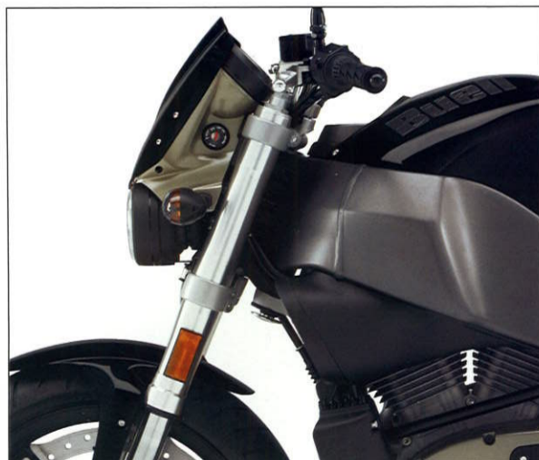
Increased rake angle (23.5°) contributes to ergonomics that feel more "relaxed" while still delivering original Lightning performance and handling.
