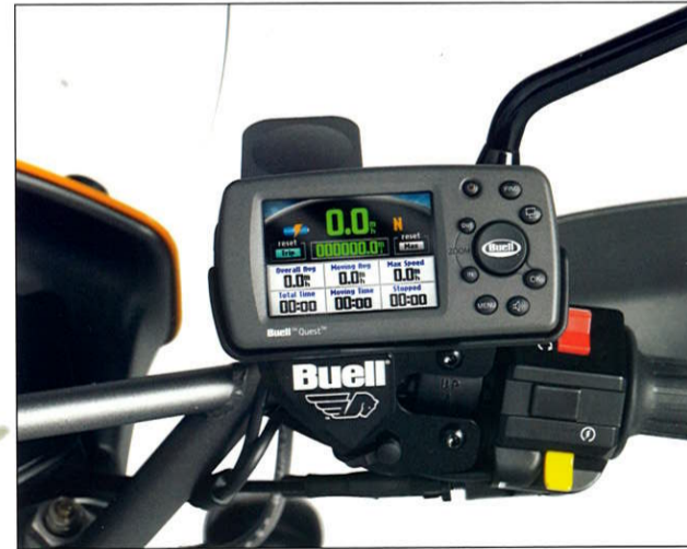
Buell Quest Waterproof Portable Navigation System has enough memory (115 MB) to plan a cross-country journey.
