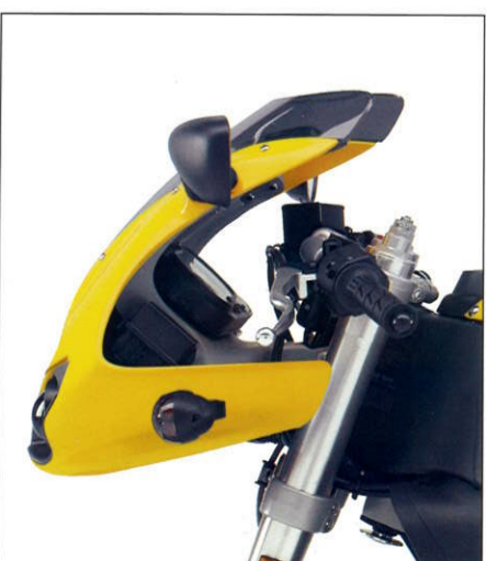
Magnesium front module cradles the reader friendly instrument cluster.
