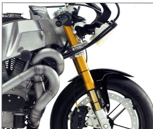
Ohlins front fork provides unmatched suspension performance.
