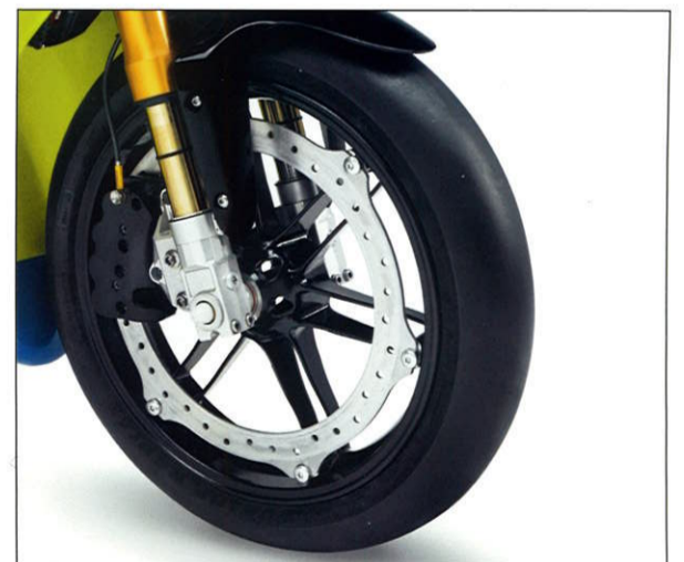
Magnesium wheels reduce the unsprung weight and keep the tires on the track.
