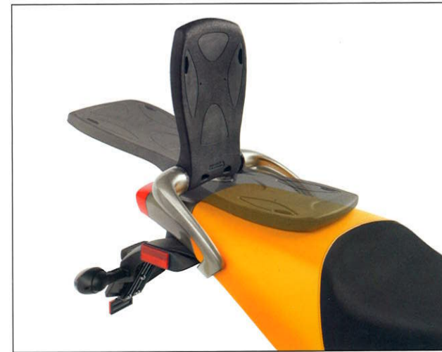
Triple Tail™: 1. Luggage rack with integrated tie-down hooks; 2. Flexible passenger backrest with grab rails; and 3. Luggage rack extending over LED taillight with passenger grab rails available.
