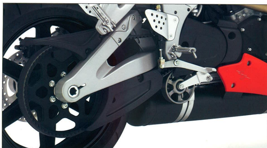
Innovative belt and pulley drive system provides immediate throttle reponse; needs no lubrication, no regular maintenance, and has no scheduled replacement.
