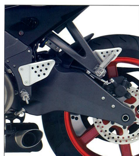
Massive aluminum swingarm is rigid and acts as oil reservoir, lowering center of gravity.
