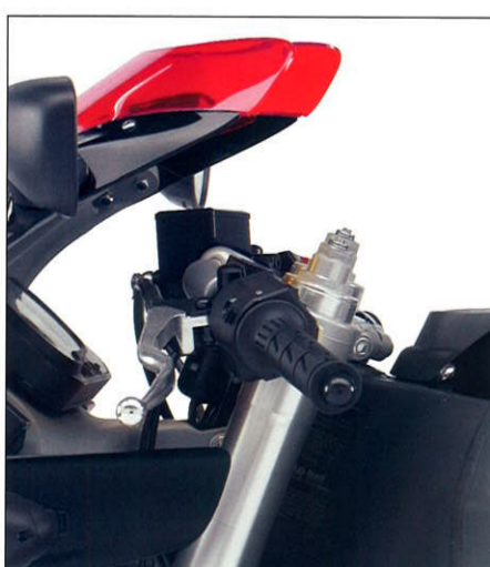
Handlebar placement tucks rider behind the front fairing.
