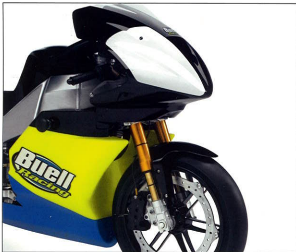
Wind-tunnel-tested carbon fiber race fairing to improve aerodynamics and reduce drag.
