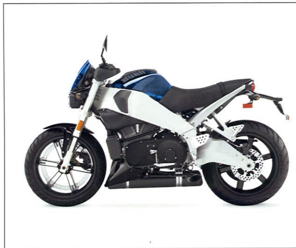
Lightning CityX XB9SX features rugged Pirelli Scorpion Sync tires and mass centralized muffler.
