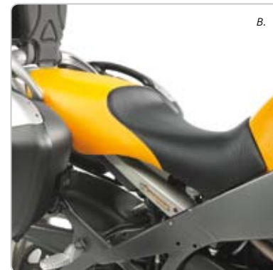
LOW SEAT HEIGHT (803MM) STOCK SEAT HEIGHT (841MM)
