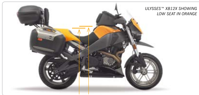
LOW SEAT HEIGHT (803MM) STOCK SEAT HEIGHT (841MM)
