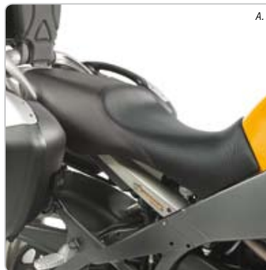
LOW SEAT HEIGHT (803MM) STOCK SEAT HEIGHT (841MM)
