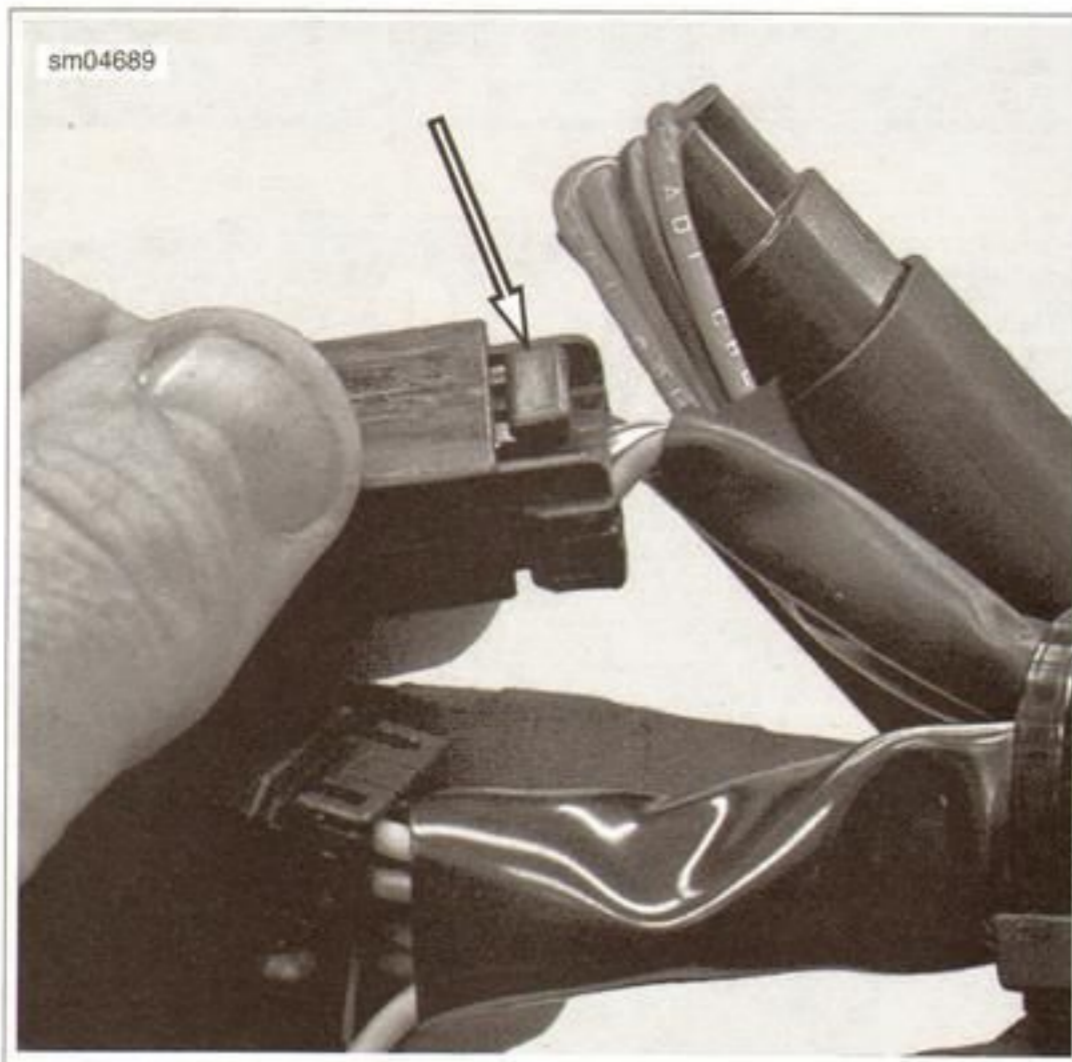
Figure 7-102. Right Handlebar Switch Connector [22] Release Button
