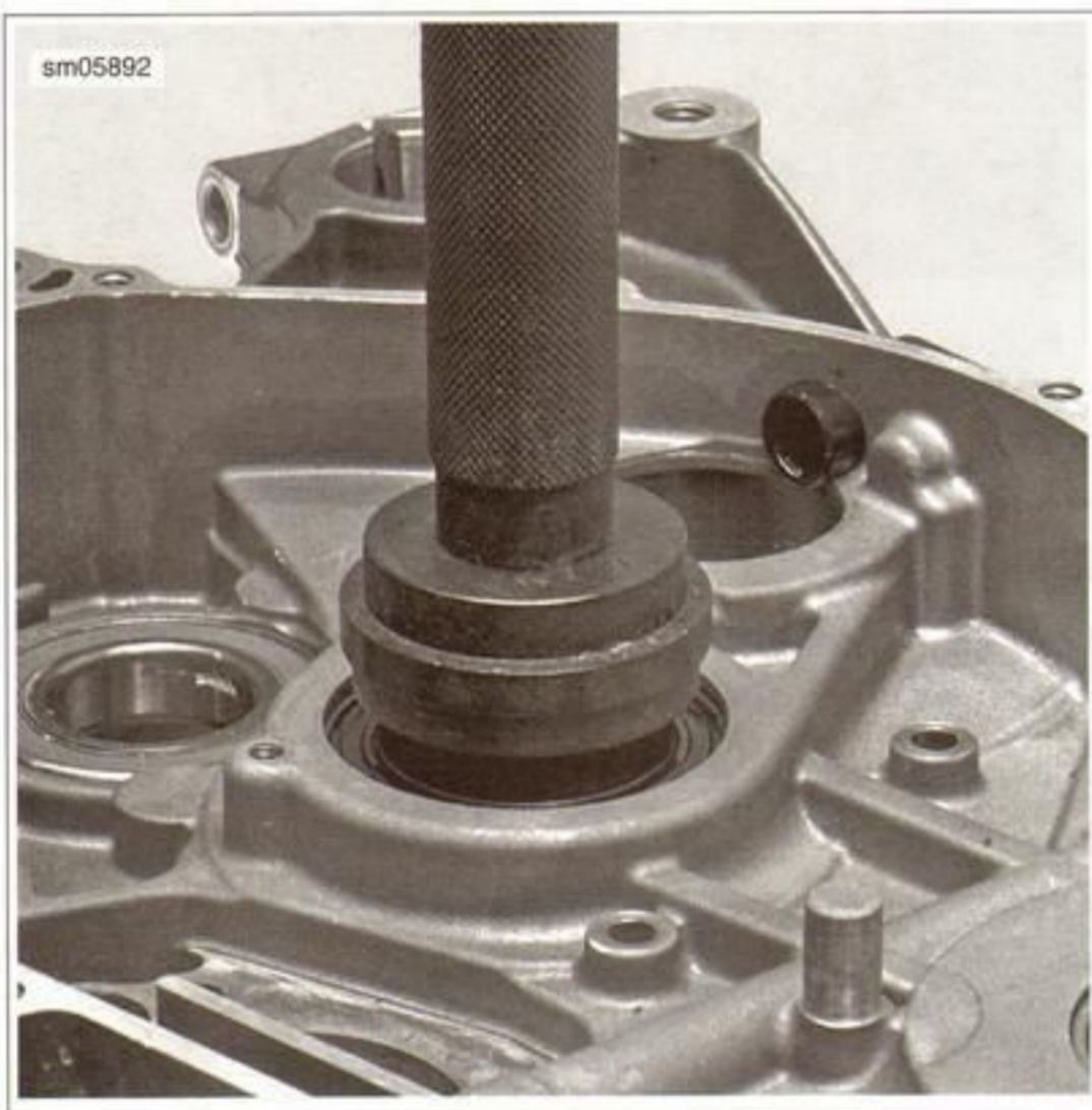
Figure 6-101. Clutch Shaft Bearing Removal: Right Case
