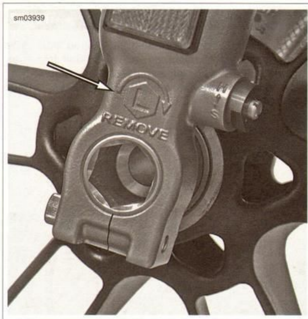
Figure 2-22. LH Thread Axle
