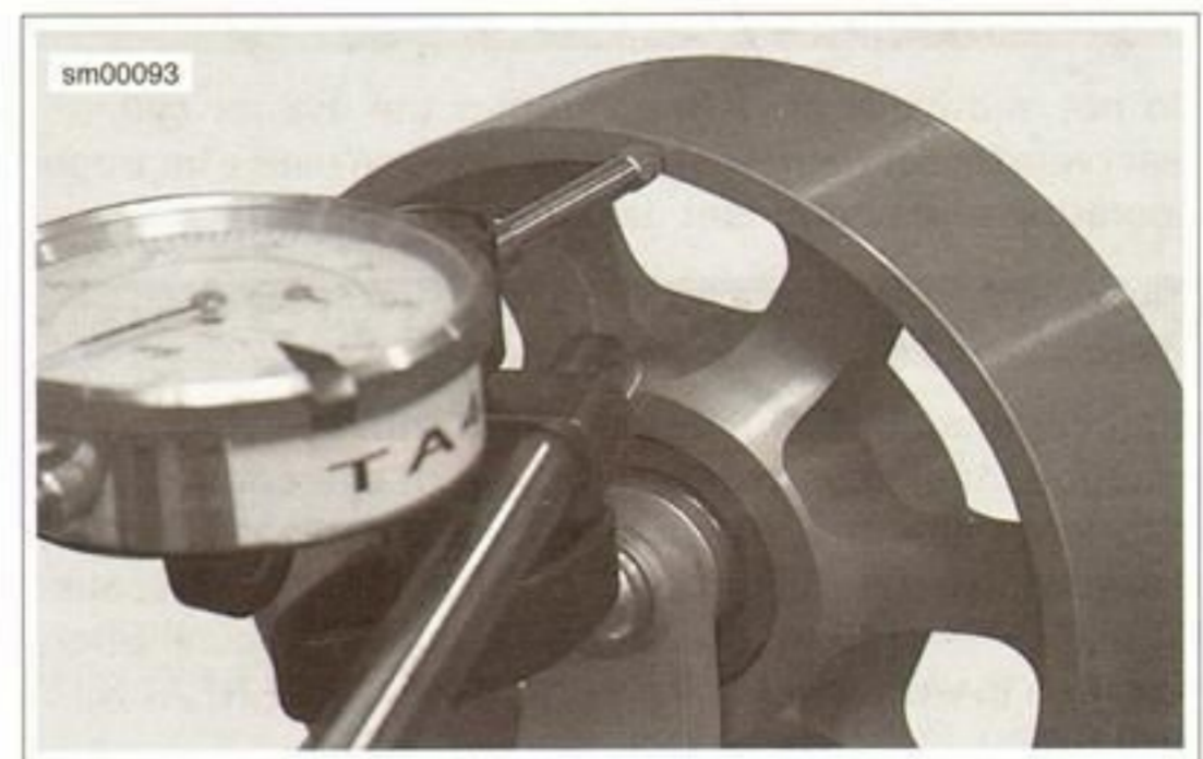
Figure 1-18. Measuring Lateral Side Play on Idler Pulley
