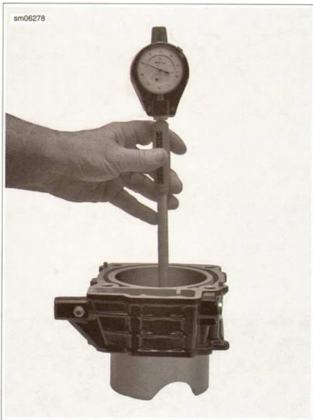
Figure 3-99. Measuring Cylinder Bore
