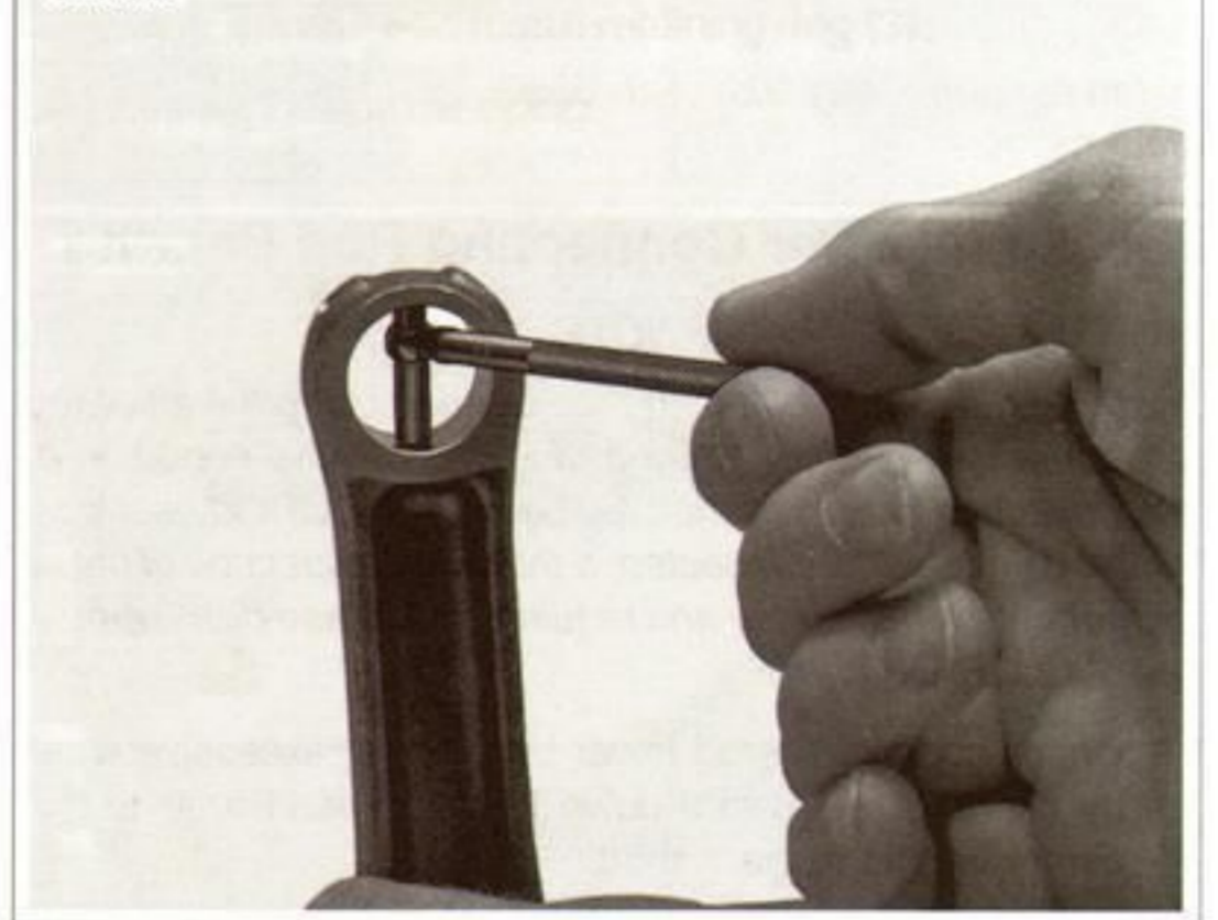
Figure 3-97. Connecting Rod Piston Pin Bore Measurement
