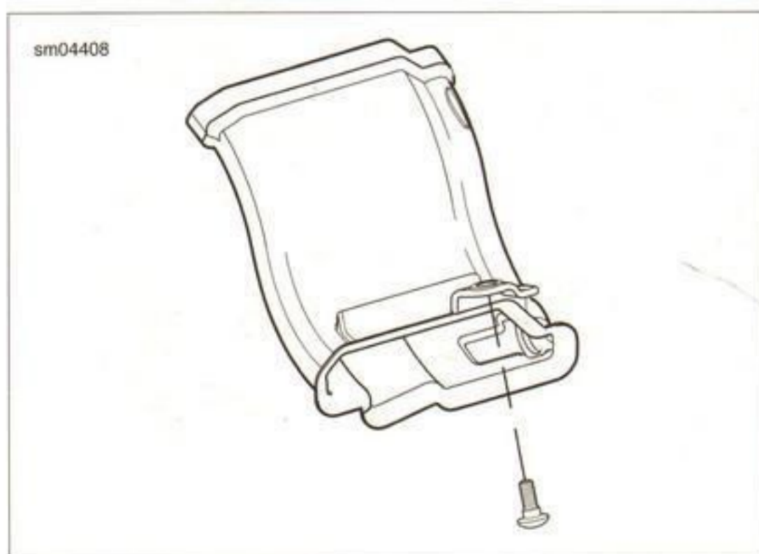
Figure 4-1. Ram Air Intake Snorkel
