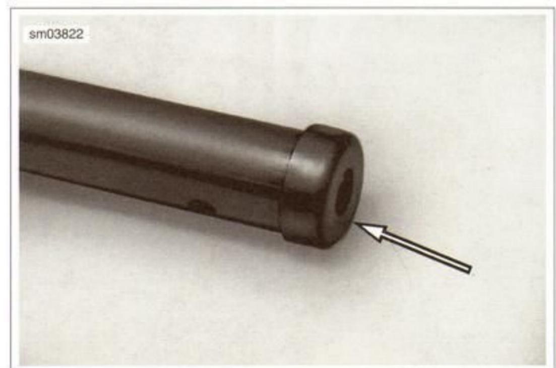
Figure 2-92. Centering Plate on Bottom of Damper Rod
