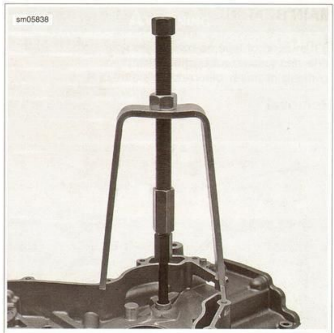
Figure 3-181. Remove the Water Pump Shaft Case Bearing
