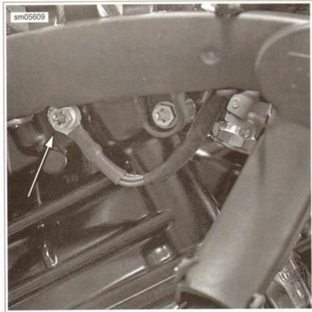
Figure 7-108. Engine Ground Connection
