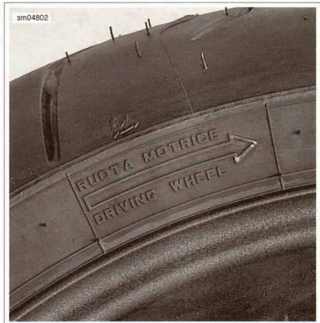
Figure 2-13. Direction of Rotation Arrow
