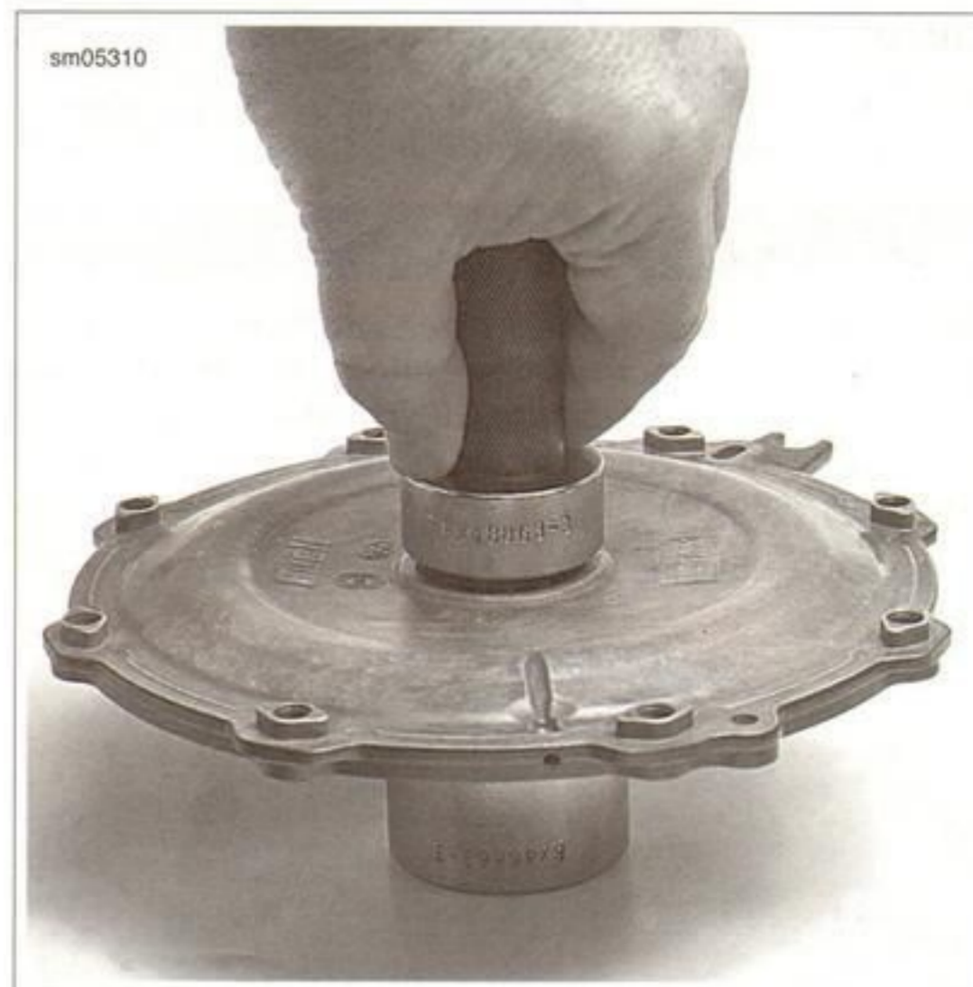
Figure 6-36. Installing the Diaphragm Oil Seal
