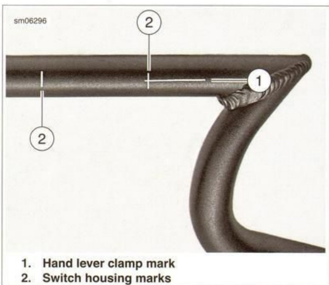
Figure 2-146. Hand Lever Clamp and Switch Housing Marks: 1125CR
