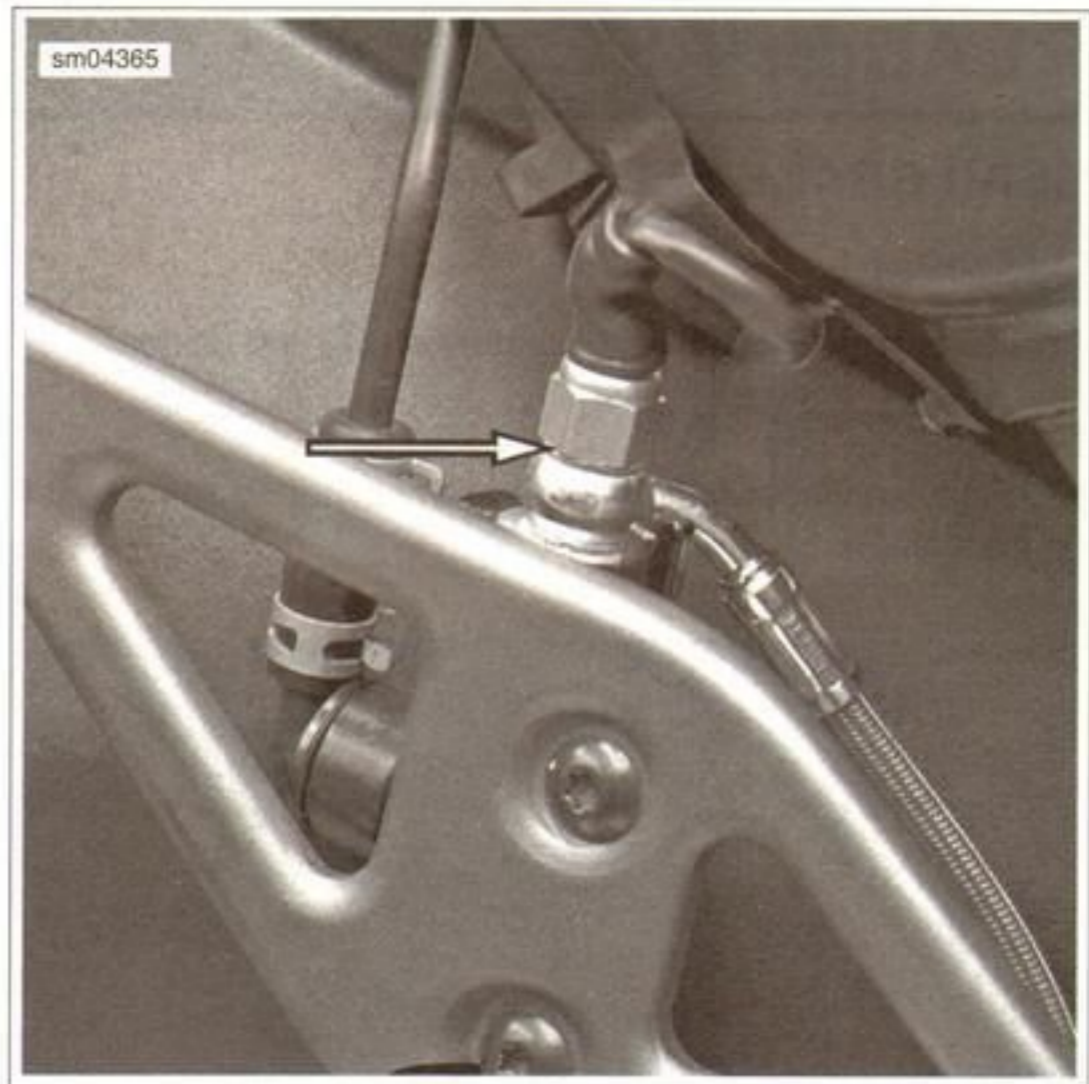
Figure 2-70. Brake Light Switch
