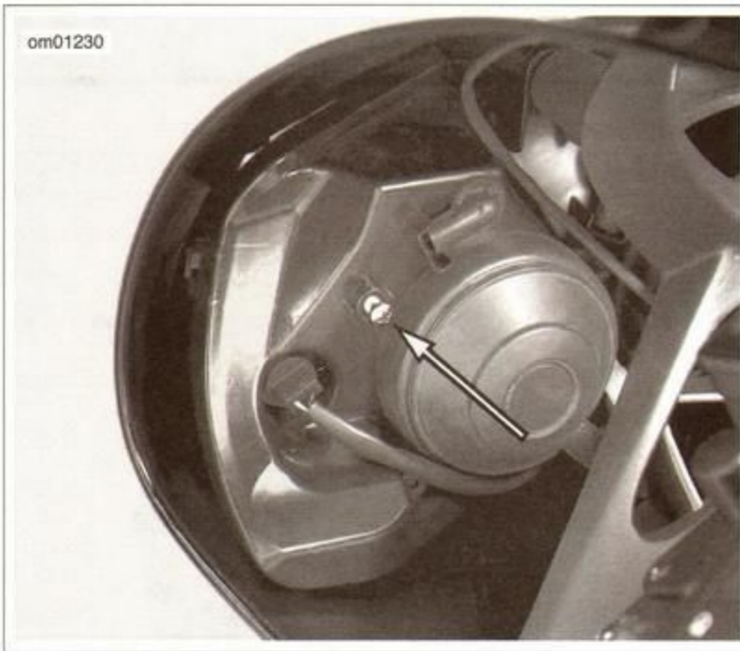
Figure 1-44. Vertical Headlamp Adjustment Screw: 1125R
