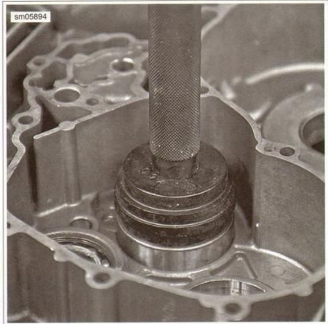
Figure 6-102. Clutch Shaft Bearing Installation: Right Case
