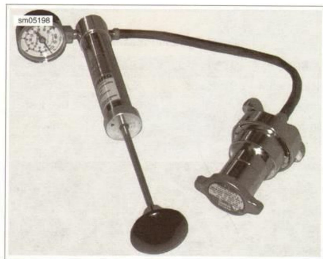
Figure 5-4. Pressure Cap Test
