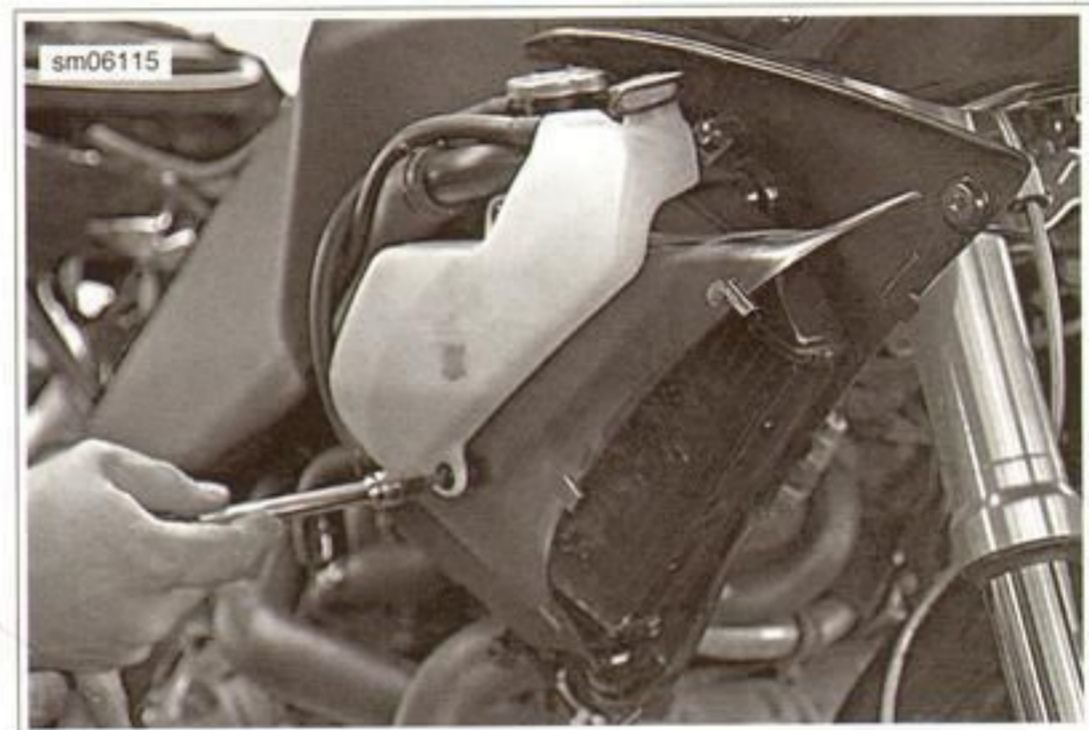
Figure 3-32. Remove Overflow Tank
