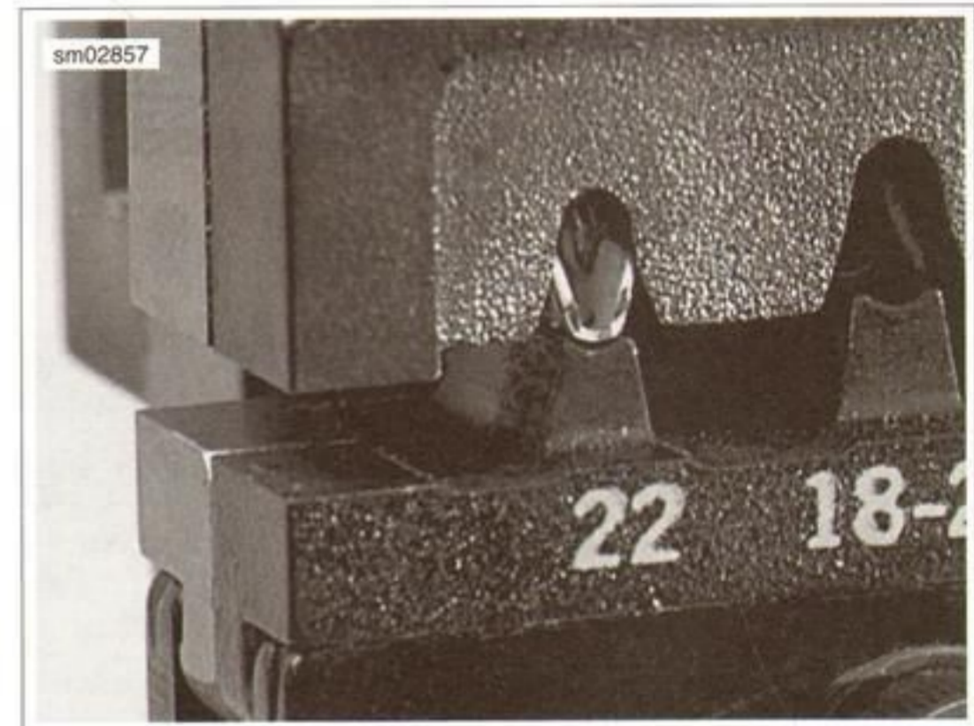
Figure A-34. Crimp Tails in Vertical Alignment between Punch and Die
