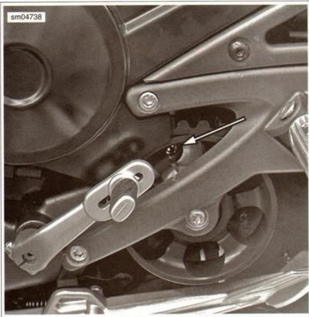
Figure 4-49. Muffler Bolt Through Idler Wheel Bracket
