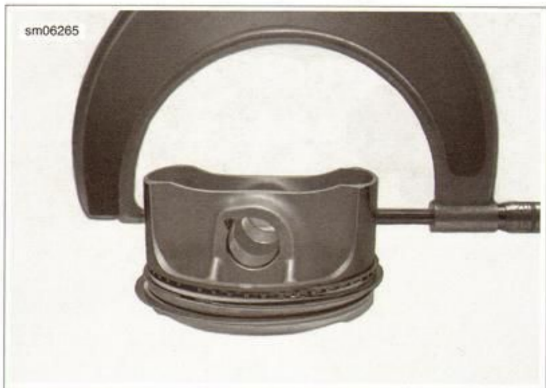
Figure 3-100. Measuring Piston Diameter
