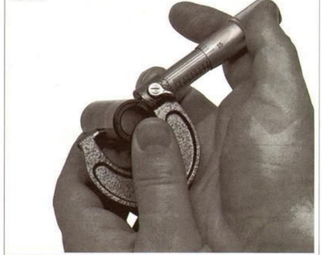
Figure 3-96. Piston Pin Diameter Measurement
