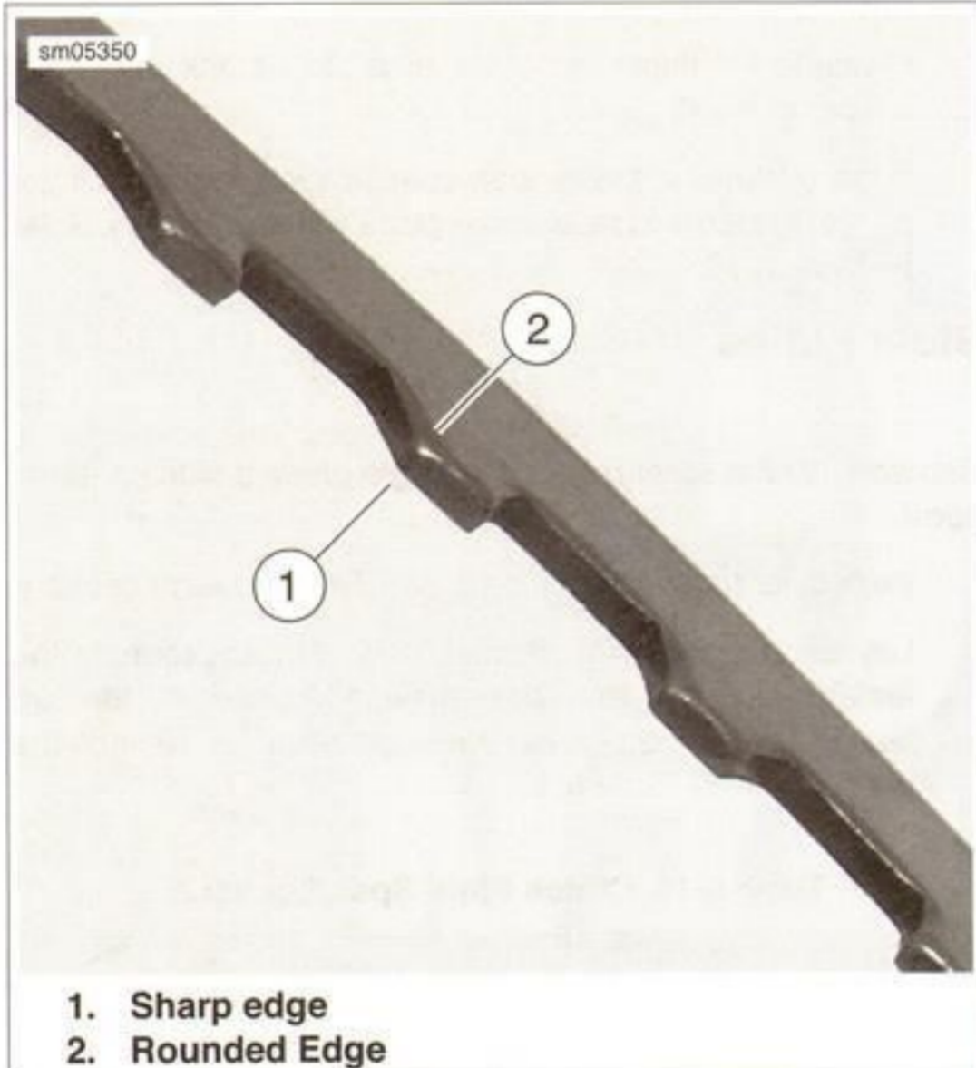
Figure 6-43. Sharp and Rounded Edge Steel Plate
