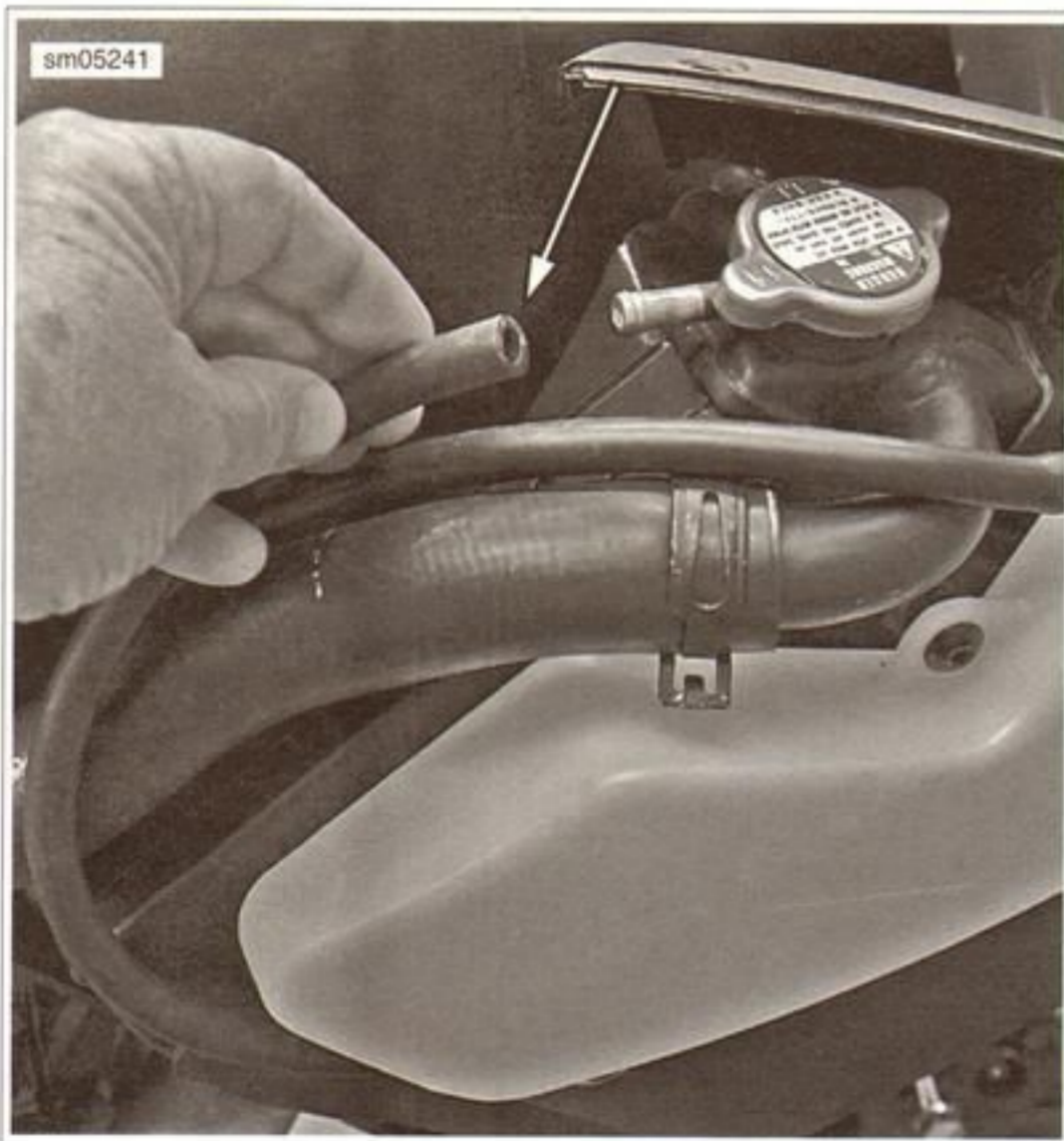
Figure 5-8. Overflow Bottle Hose
