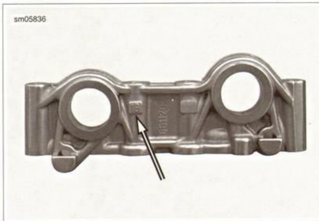
Figure 3-77. Camshaft Bracket Identification
