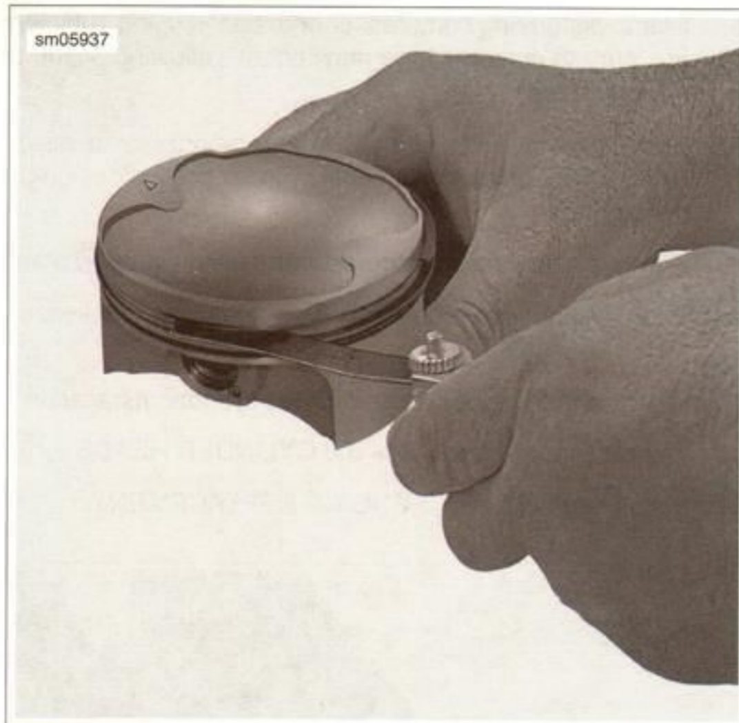
Figure 3-103. Ring Side Clearance
