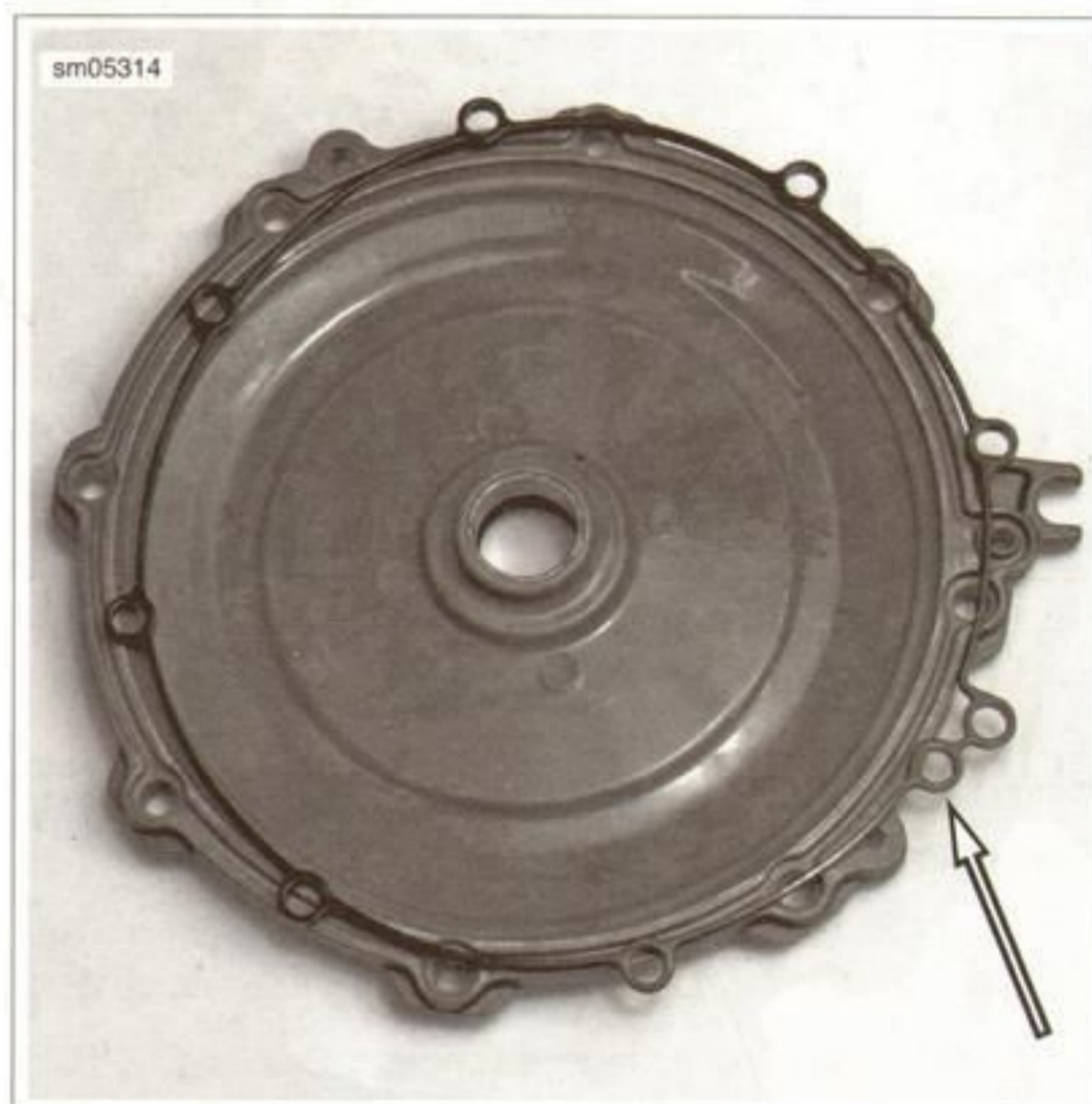
Figure 6-37. Gasket to Cover Matching Features
