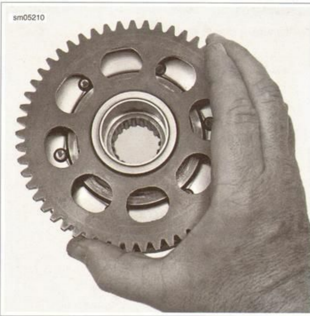
Figure 7-37. Rotate Starter Gear to Fit Sprag Clutch
