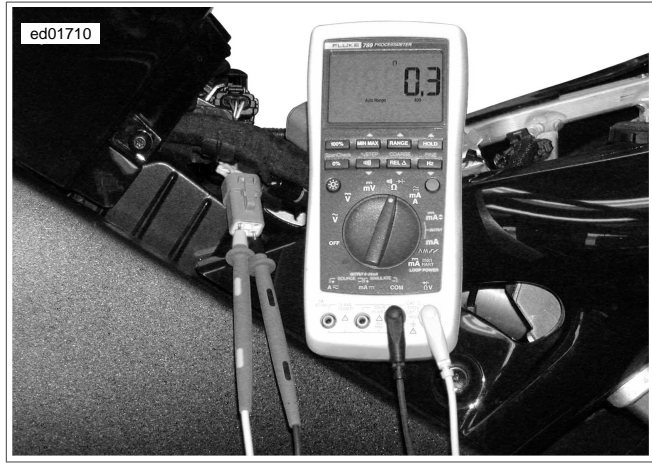
Figure 3-18. Check for Stator Resistance (typical)
