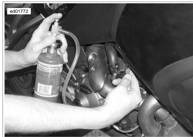
Figure 1-26. Checking for Leaks
