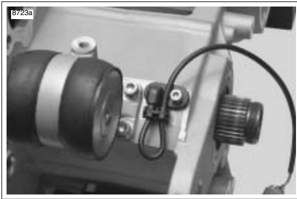
Figure 3-30. Rear Isolator and Mounting Hardware
