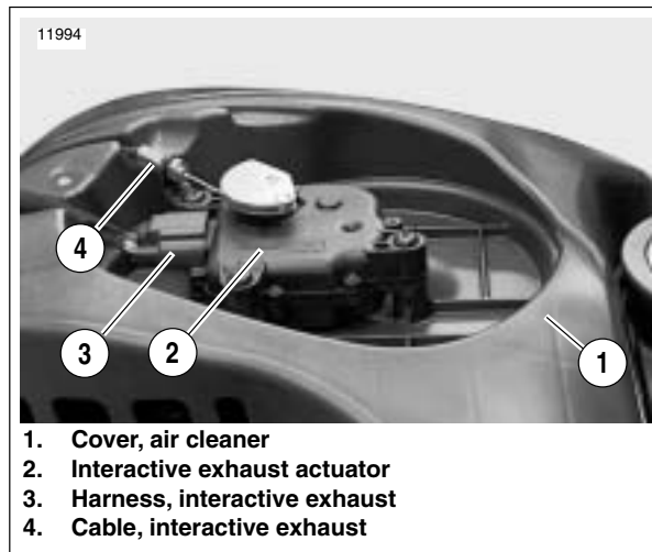
Figure 1-111. Air Cleaner Cover, Interactive Exhaust Components
