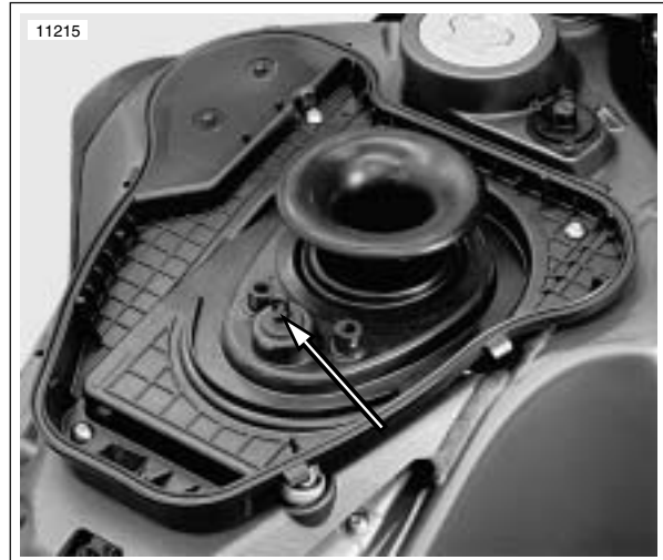
Figure 4-78. Intake Air Temperature Sensor Installed
