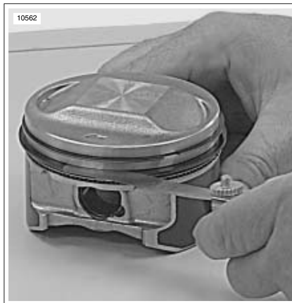
Figure 3-95. Measuring Ring Clearance in Groove
