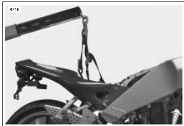
Figure 3-40. Supporting Vehicle for Assembly (Typical)
