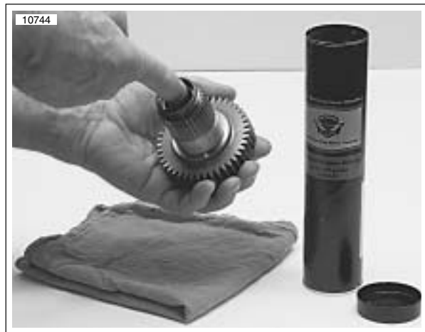
Figure 6-76. Lubricating Main Drive Gear Needle Bearings
