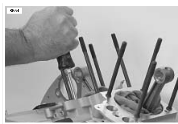
Figure 3-132. Checking Cam Gear End Play
