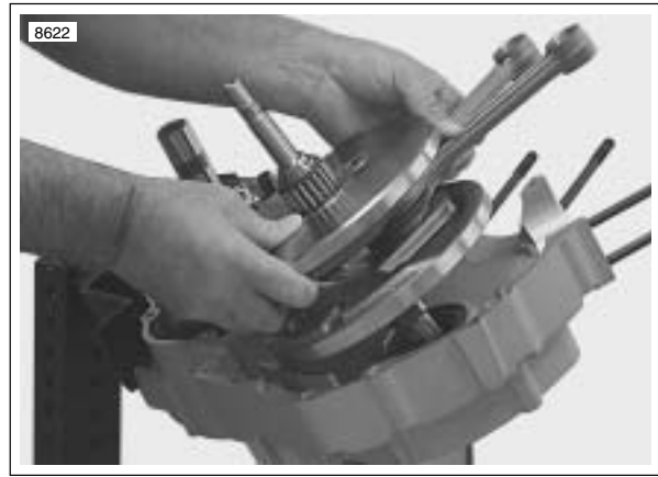
Figure 3-136. Removing Flywheels from Left Crankcase
