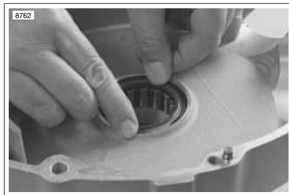
Figure 3-140. Removing Sprocket Shaft Bearing Retaining Ring
