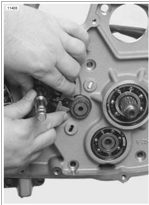
Figure 6-49. Removing Shifter Shaft Assembly
