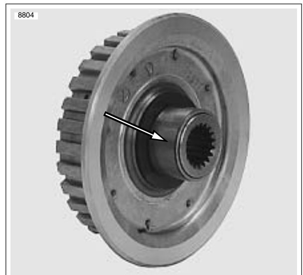
Figure 6-28. Clutch Hub Bearing Race
