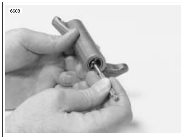
Figure 3-66. Measuring Rocker Arm Bushing Inner Diameter
