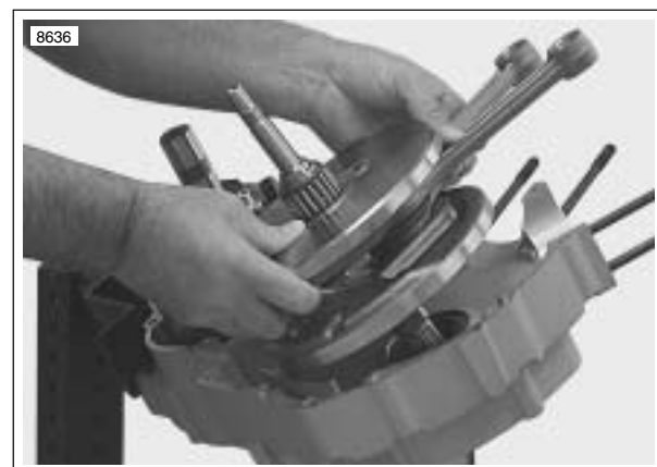
Figure 6-54. Removing Flywheels from Left Case Half
