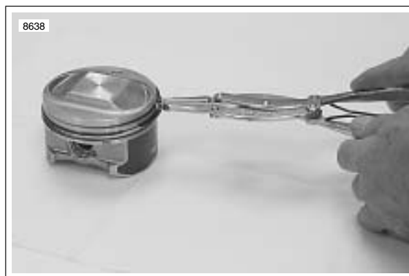
Figure 3-88. Removing Piston Rings
