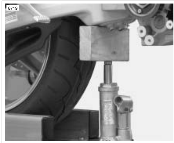
Figure 3-37. Supporting the Swingarm (Typical)
