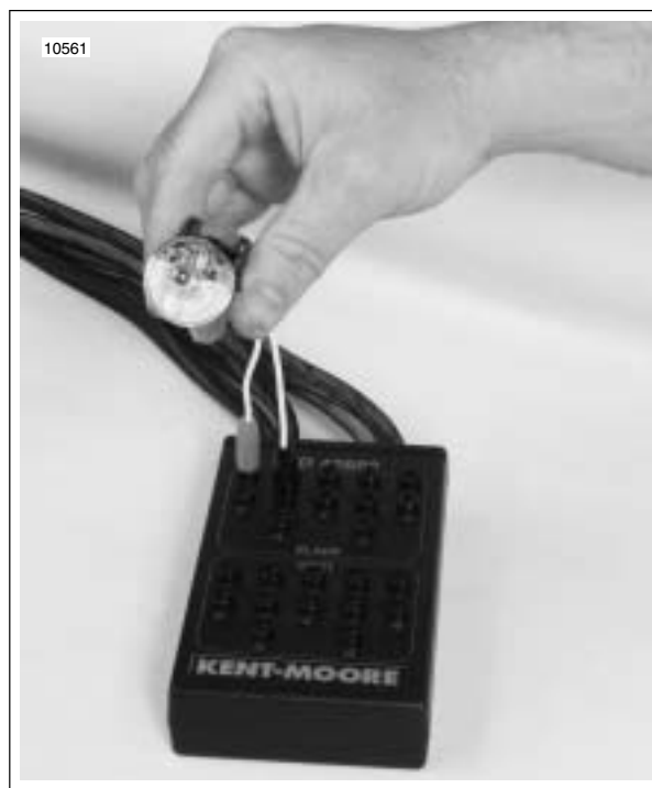
Figure 4-48. Testing Ignition Coil Connectors
