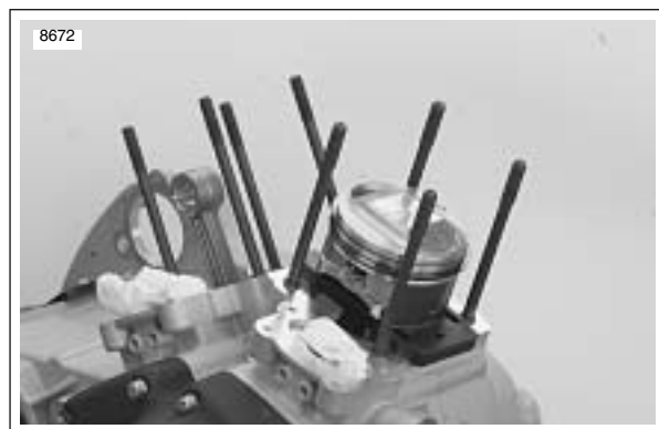
Figure 3-104. Piston Support Plate
