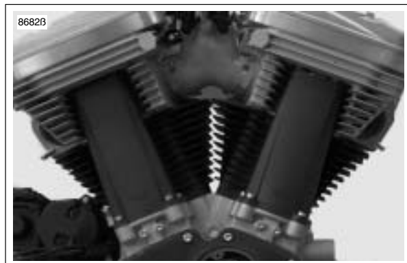
Figure 3-79. Push Rod Locations
