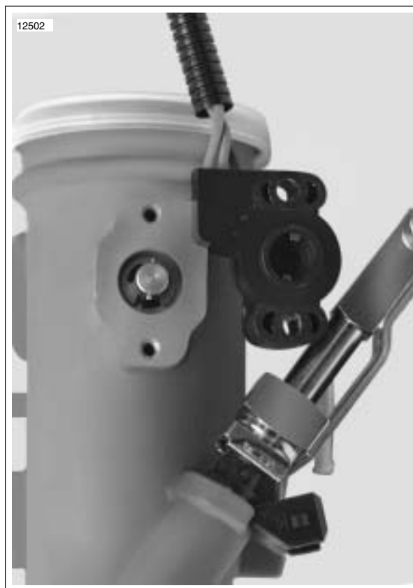
Figure 4-80. Throttle Position Sensor
