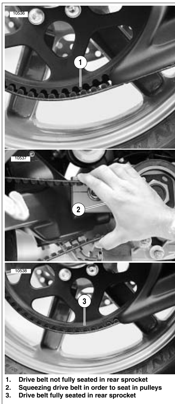
Figure 6-42. Seating Drive Belt Into Pulley Teeth
