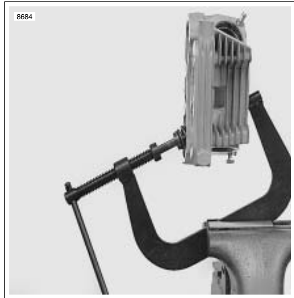
Figure 3-78. Valve Spring Compressor (Part No. HD-34736B)
