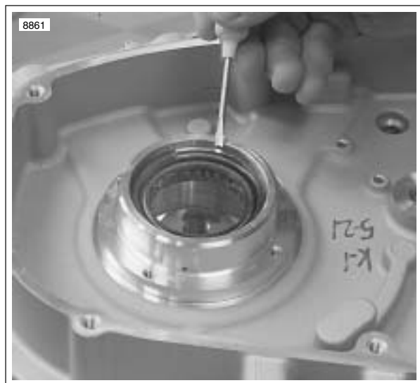
Figure 3-139. Sprocket Shaft Seal Retaining Ring
