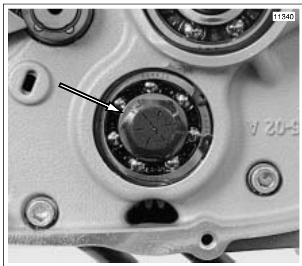
Figure 6-46. Hex Fastener Countershaft Retainer
