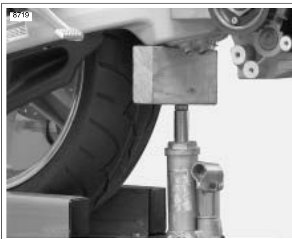
Figure 3-23. Supporting the Swingarm (Typical)
