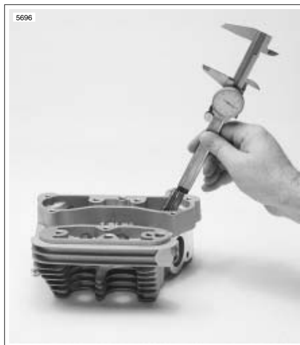
Figure 3-67. Measuring Valve Stem Protrusion
