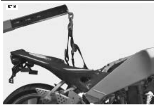
Figure 3-22. Supporting Vehicle for Disassembly (Typical)
