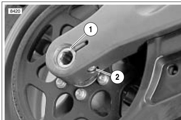
Figure 6-41. Rear Wheel Mounting, Right Side
