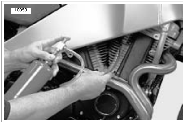
Figure 4-110. Checking for Intake Leak
