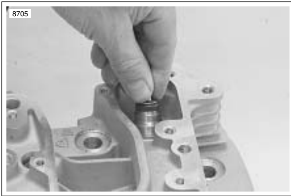
Figure 3-77. Valve Seal and Lower Collar Assembly Installation
