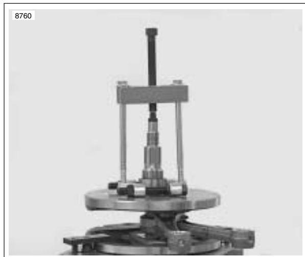
Figure 3-138. Removing Sprocket Shaft Inner Bearing Race
