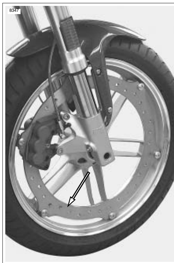
Figure 1-15. Front Brake Rotor
