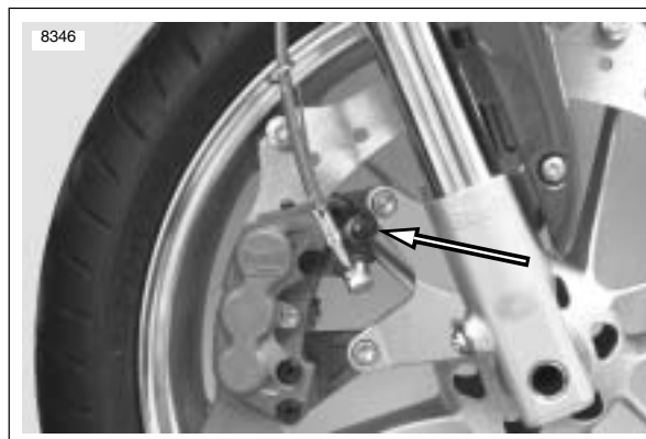
Figure 1-8. Front Caliper Bleeder Valve
