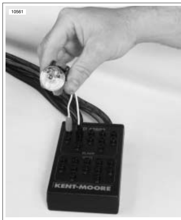
Figure 4-50. Testing Ignition Coil Connectors
