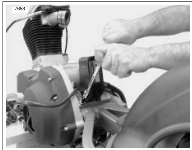
Figure 3-17. Rear Engine Mount
