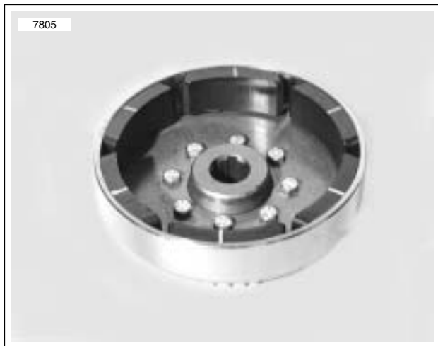
Figure 7-52. Rotor Assembly
