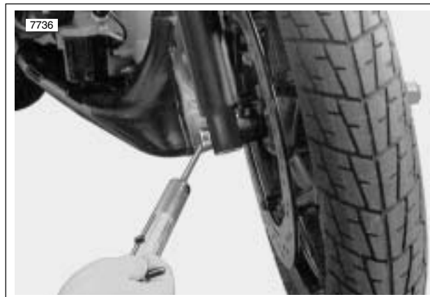
Figure 1-33. Steering Head Bearing Check
