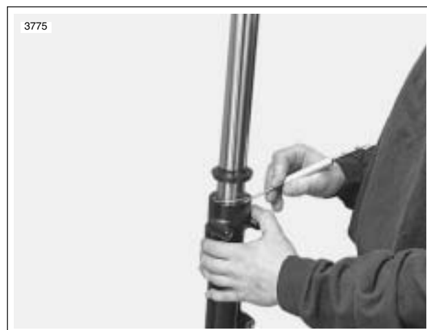
Figure 2-74. Removing Dust Seal
