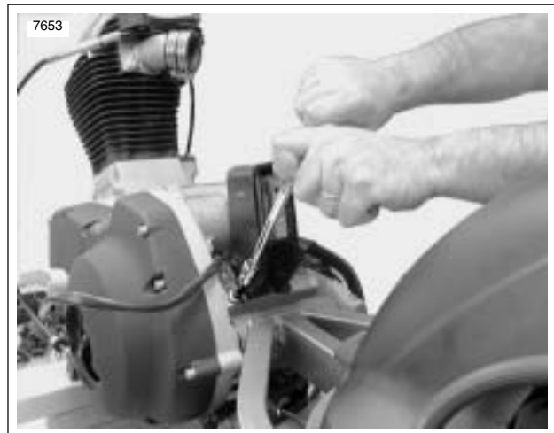
Figure 3-24. Rear Engine Mount
