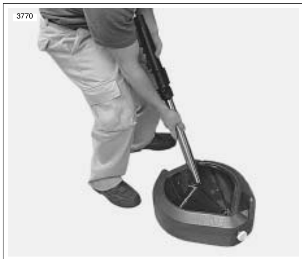
Figure 1-30. Pumping Fork Oil
