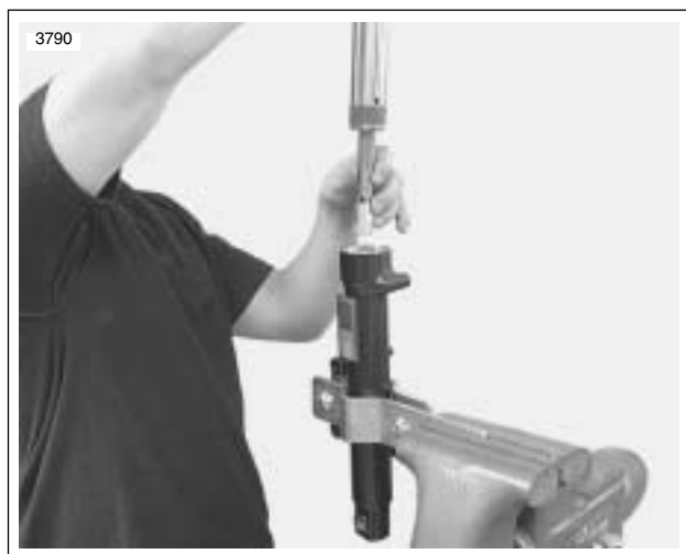
Figure 2-83. Installing Slider Tube
