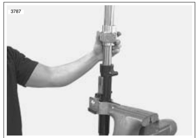
Figure 2-89. Fork Seal Driver
