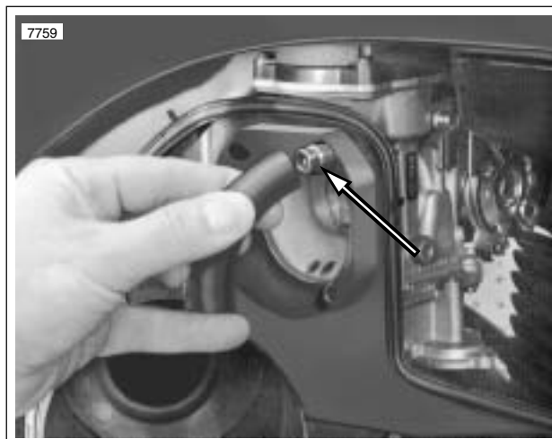
Figure 1-38. Fix Hose End Onto Allen Head Screw
