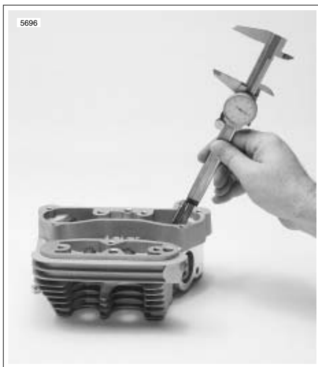
Figure 3-55. Measuring Valve Stem Protrusion
