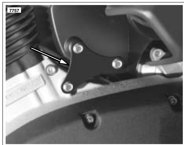
Figure 1-37. Air Cleaner Mounting Bracket (left side)
