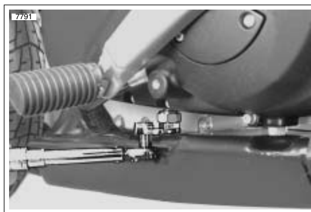
Figure 1-24. Tightening Chain Limiting Screw
