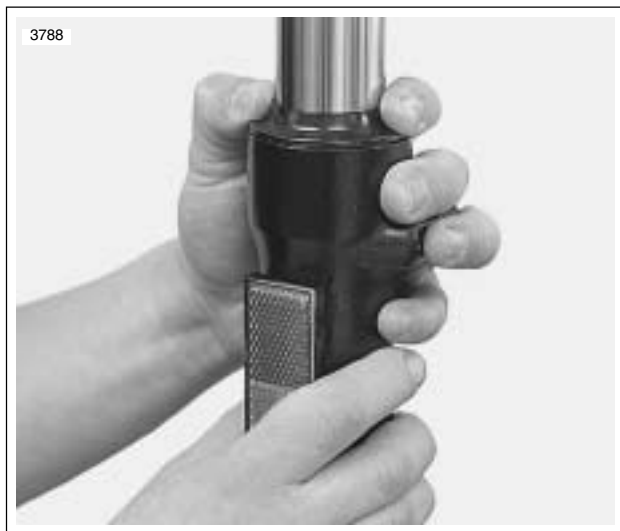
Figure 2-91. Install New Dust Seal
