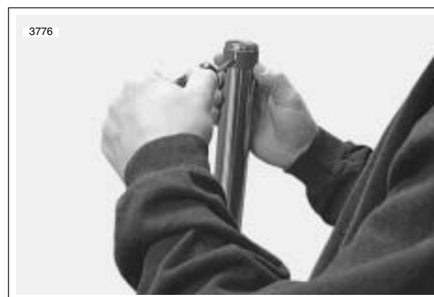
Figure 2-76. Removing Slide Bushing
