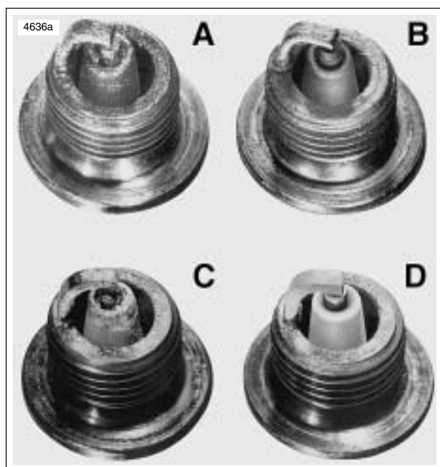
Figure 1-35. Typical Spark Plug Deposits
