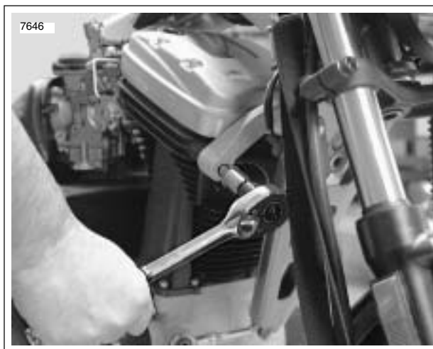
Figure 3-2. Cylinder Head Bolts
