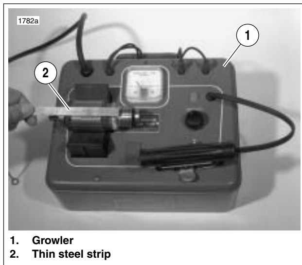
Figure 5-20. Shorted Armature Test Using Growler
