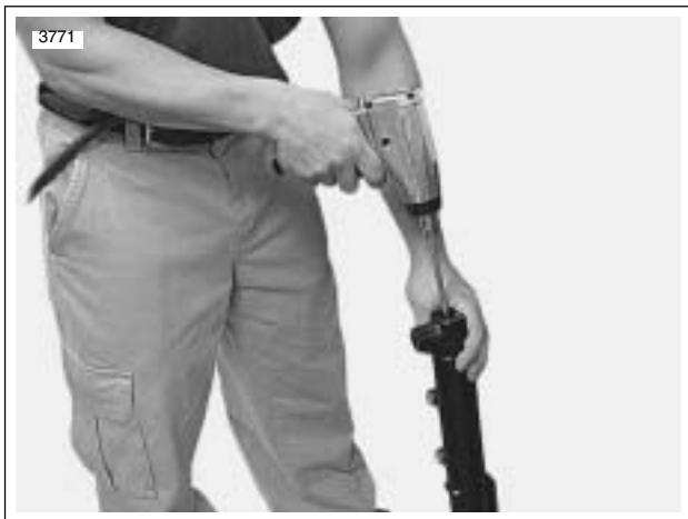
Figure 2-72. Removing Center Bolt
