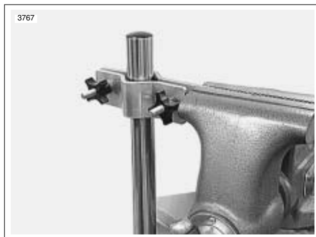
Figure 1-26. Clamping the Fork
