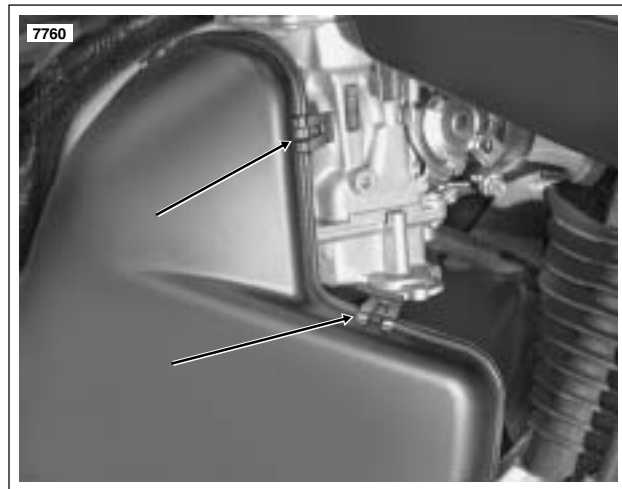
Figure 1-36. Release Air Box Cover Latches
