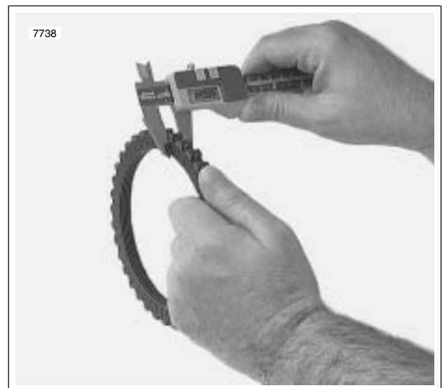
Figure 6-18. Measuring Friction Plates
