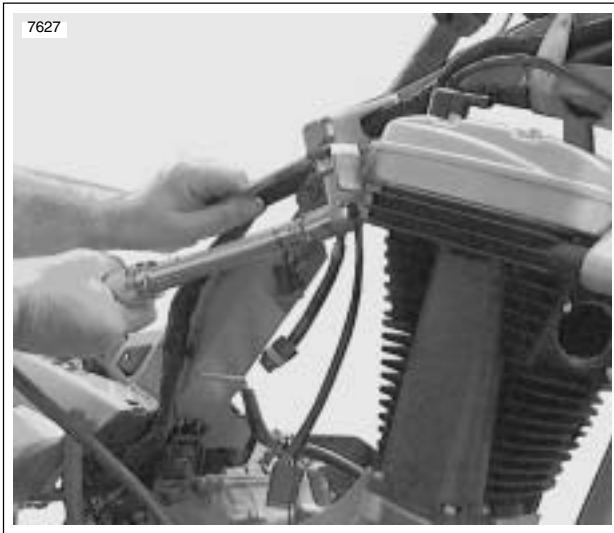
Figure 3-38. Install Top Rear Tie Bar
