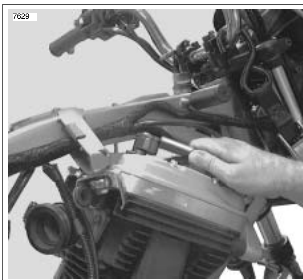
Figure 3-1. Remove Crankcase Breather Hose
