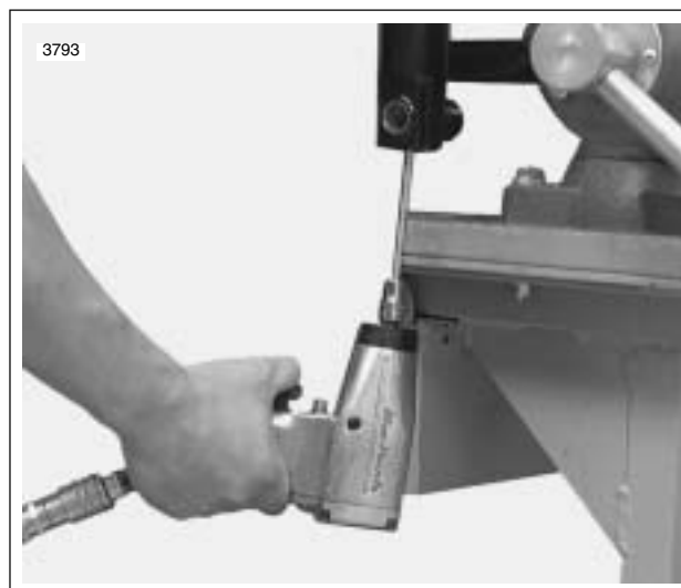
Figure 2-85. Install Center Bolt
