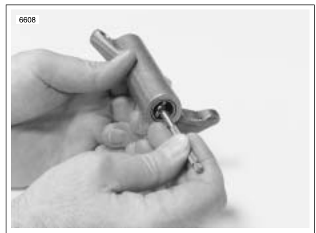
Figure 3-54. Measuring Rocker Arm Bushing Inner Diameter
