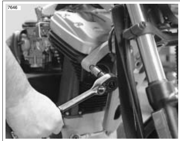
Figure 3-40. Cylinder Head Bolt
