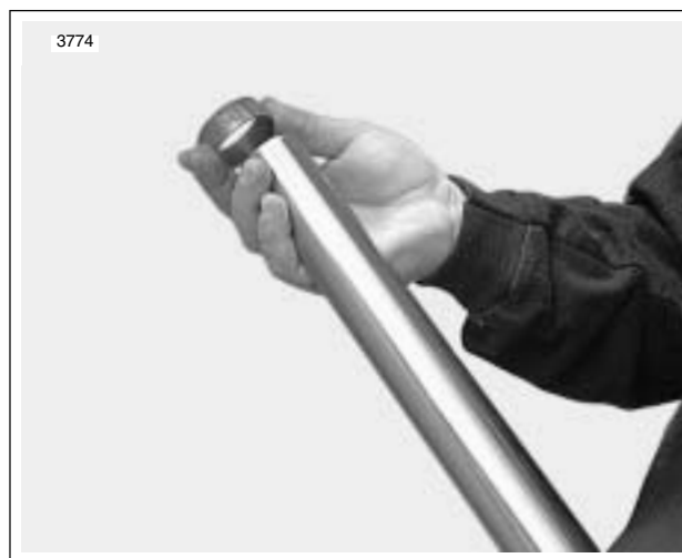
Figure 2-86. Install Guide Bushing
