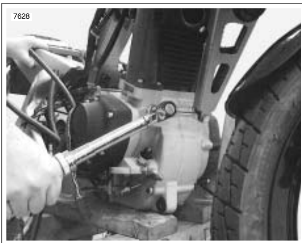
Figure 3-39. Install Front Tie Bar
