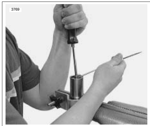
Figure 2-93. Compressing Spring Seat to Install Stopper Ring
