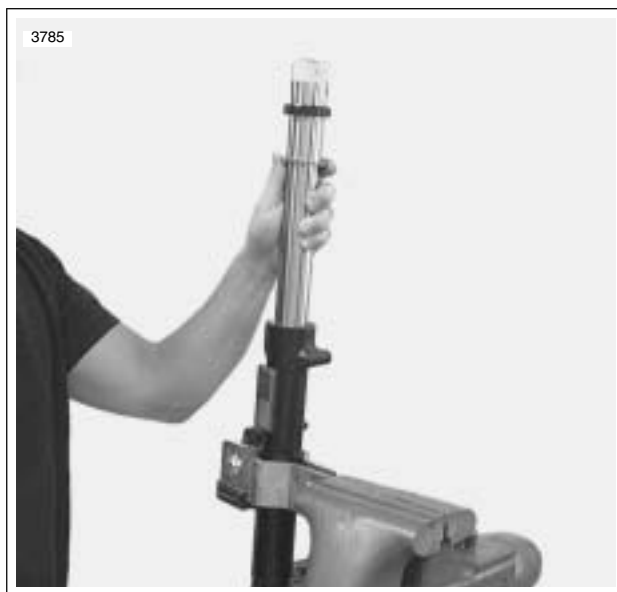
Figure 2-88. Oil Seal and Backup Ring
