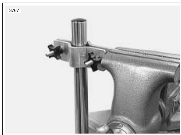
Figure 2-67. Clamping the Fork
