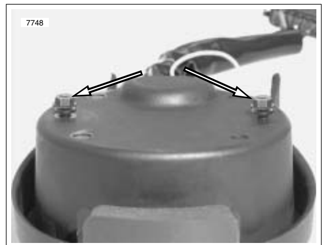
Figure 7-81. Speedometer Fasteners
