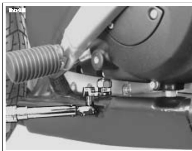
Figure 6-6. Torquing Chain Limiting Screw
