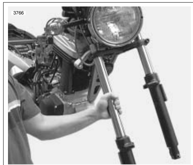
Figure 2-66. Front Fork Removal
