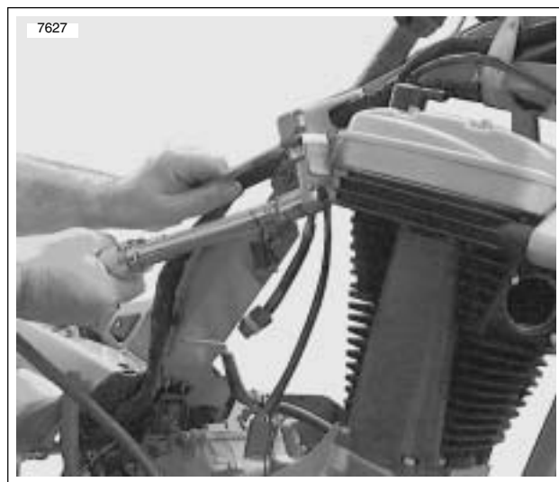
Figure 3-4. Remove Top Rear Tie Bar
