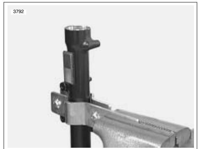
Figure 2-82. Clamping the Slider Assembly
