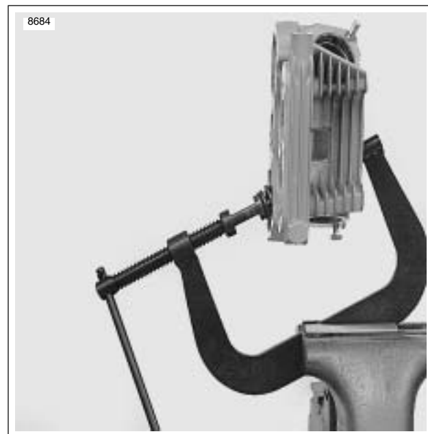
Figure 3-48. Valve Spring Compressor (Part No. HD-34736B)
