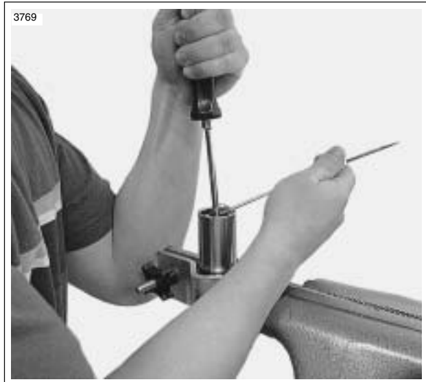
Figure 1-31. Compressing Spring Seat
