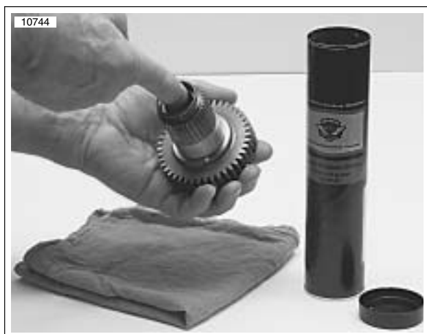
Figure 6-41. Lubricating Main Drive Gear Needle Bearings
