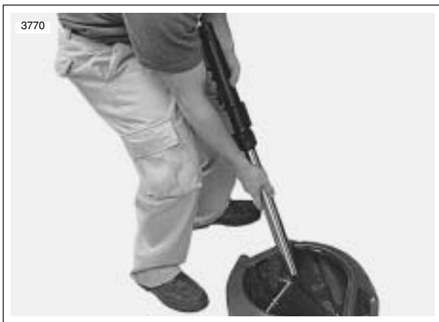
Figure 2-71. Pumping Fork Oil
