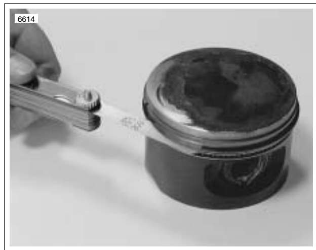
Figure 3-79. Measuring Ring Clearance in Groove
