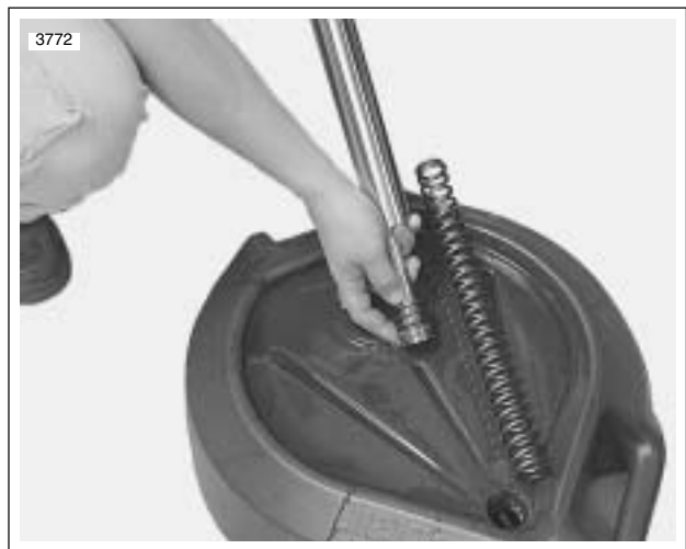
Figure 2-73. Removing Damper
