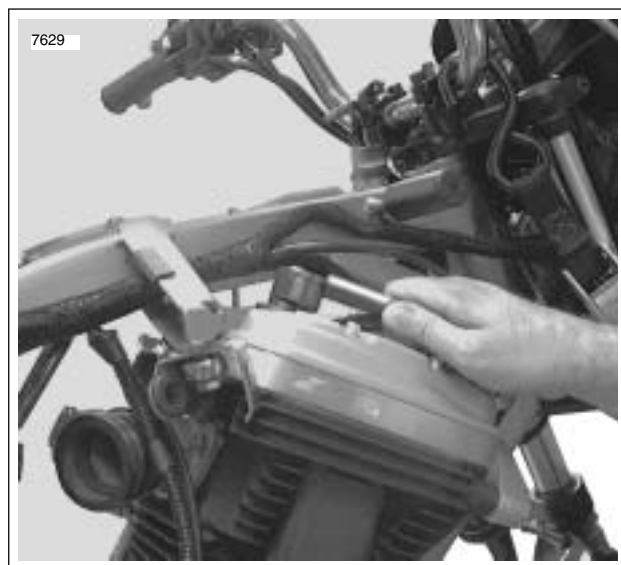
Figure 3-42. Install Crankcase Breather Hose
