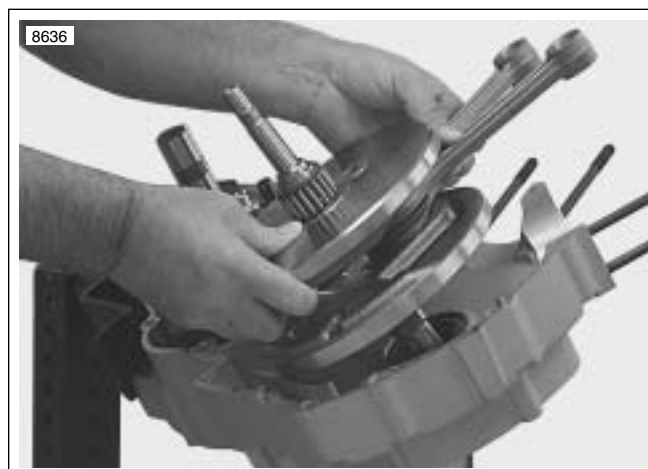
Figure 6-54. Removing Flywheels from Left Case Half
