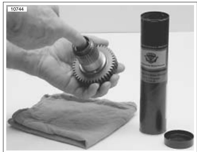
Figure 6-75. Lubricating Main Drive Gear Needle Bearings
