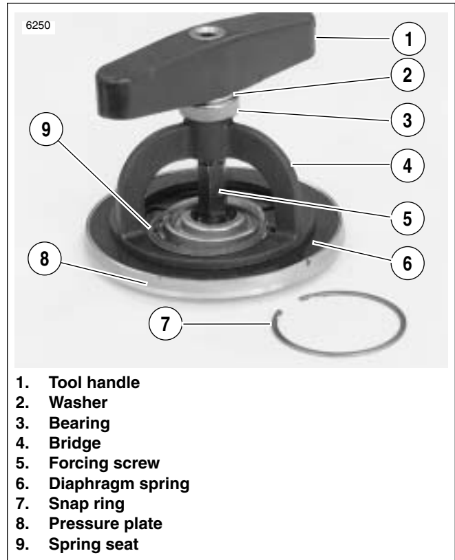
Figure 6-14. Pressure Plate Assembly
