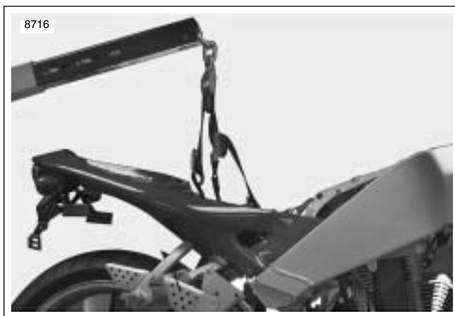
Figure 3-23. Supporting Vehicle for Disassembly (Typical)
