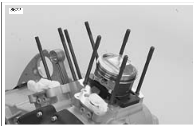
Figure 3-105. Piston Support Plate
