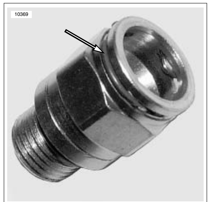
Figure 3-109. Oil Line Fitting with Spring Clip
