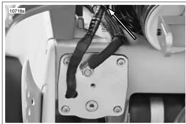
Figure 4-101. Fuel Pump Connector [86] (swingarm removed for illustration)
