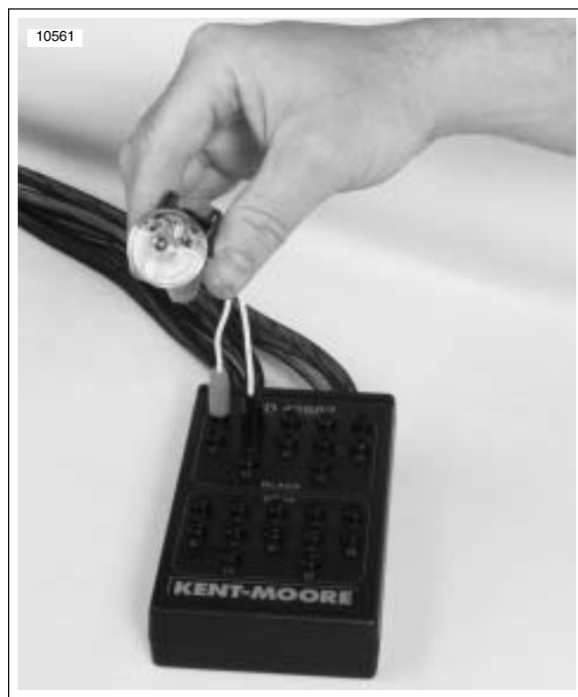
Figure 4-50. Testing Ignition Coil Connectors
