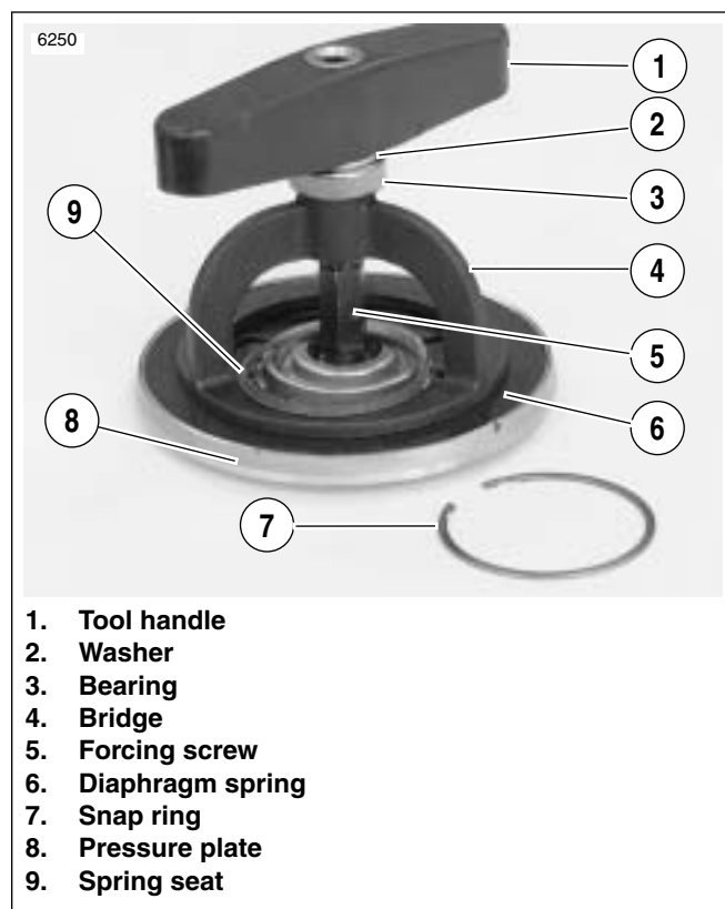
Figure 6-22. Pressure Plate Assembly
