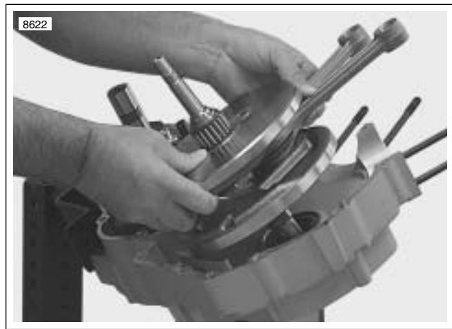
Figure 3-136. Removing Flywheels from Left Crankcase
