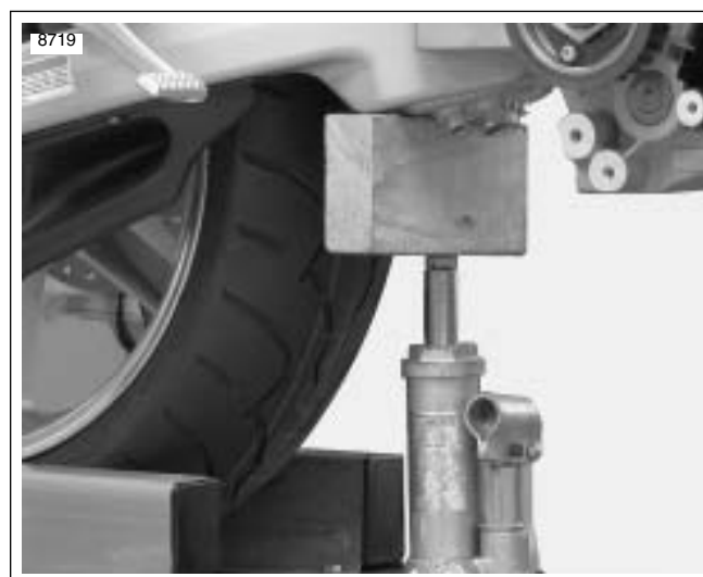
Figure 3-25. Supporting the Swingarm (Typical)
