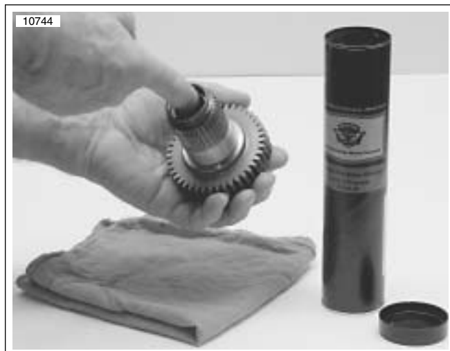
Figure 6-75. Lubricating Main Drive Gear Needle Bearings
