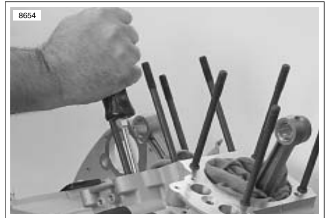
Figure 3-132. Checking Cam Gear End Play
