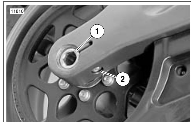
Figure 6-41. Rear Wheel Mounting, Right Side
