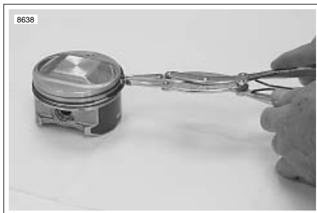
Figure 3-89. Removing Piston Rings
