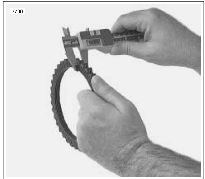
Figure 6-17. Measuring Friction Plates
