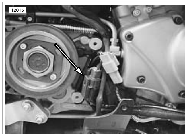
Figure 4-66. Cam Position Sensor Connector [14]
