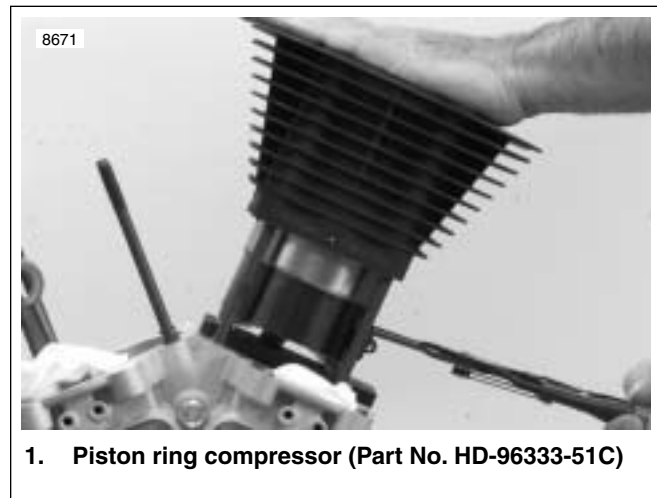
Figure 3-106. Compressing Piston Rings
