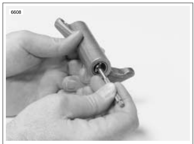
Figure 3-67. Measuring Rocker Arm Bushing Inner Diameter
