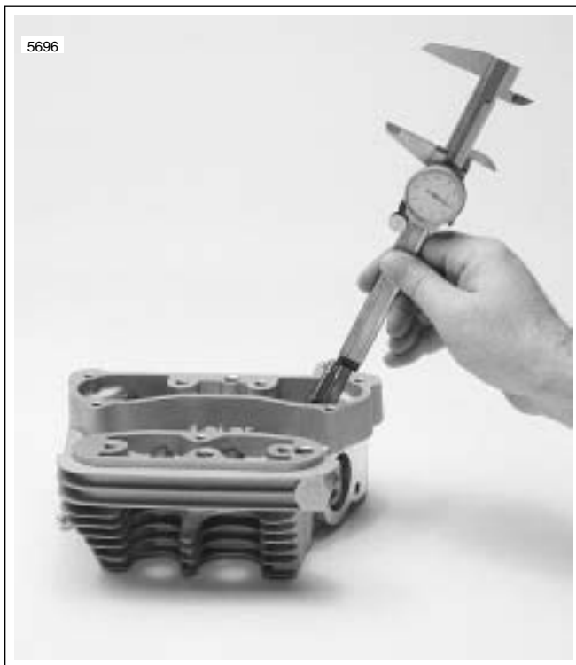
Figure 3-68. Measuring Valve Stem Protrusion
