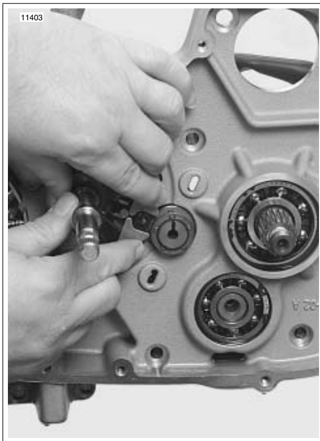
Figure 6-97. Installing Shifter Shaft Assembly
