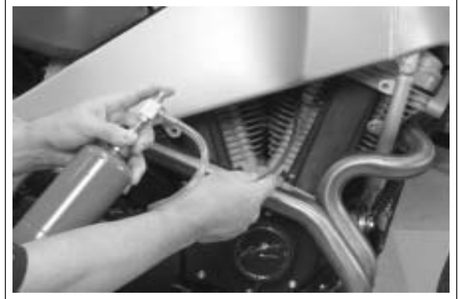
Figure 4-110. Checking for Intake Leak
