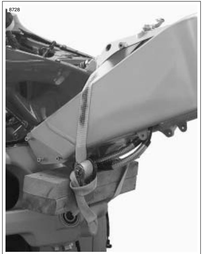
Figure 3-32. Securing Vehicle for Relocation (Typical)
