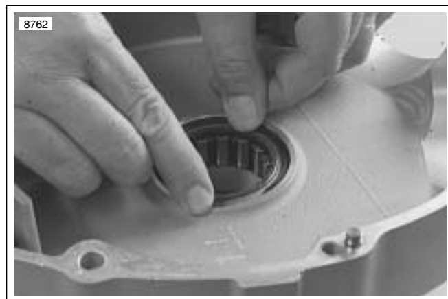
Figure 3-140. Removing Sprocket Shaft Bearing Retaining Ring
