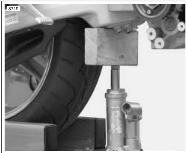
Figure 3-38. Supporting the Swingarm (Typical)
