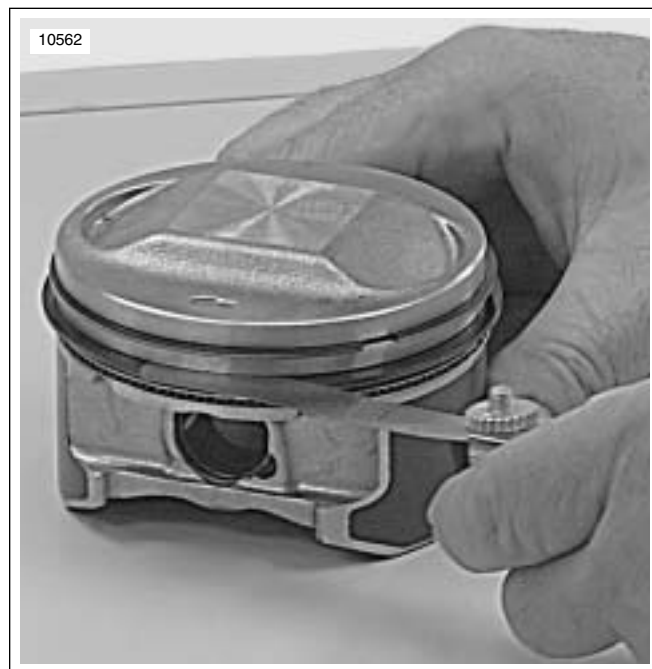
Figure 3-96. Measuring Ring Clearance in Groove
