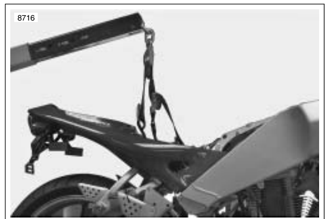
Figure 3-41. Supporting Vehicle for Assembly (Typical)
