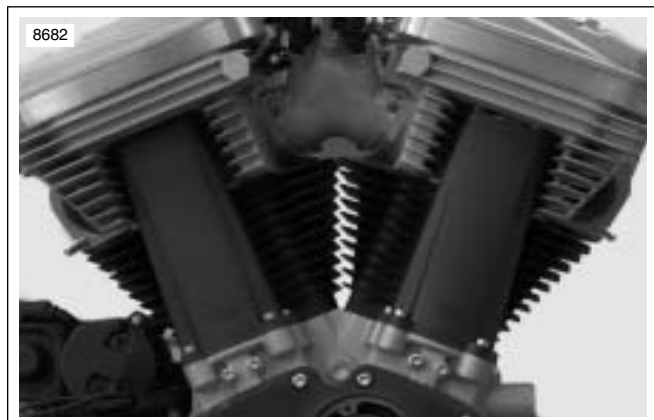
Figure 3-80. Push Rod Locations
