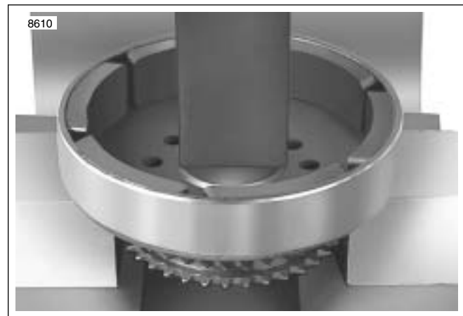
Figure 7-33. Removing Rotor From Sprocket
