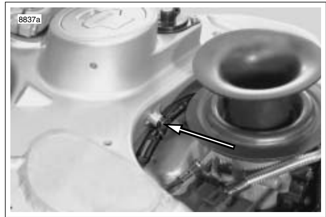
Figure 7-78. Wire Harness Clip
