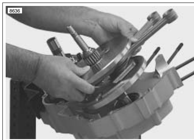
Figure 6-54. Removing Flywheels from Left Case Half
