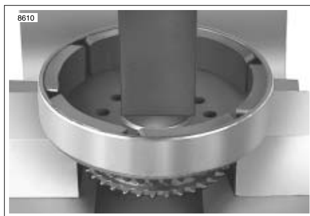
Figure 7-33. Removing Rotor From Sprocket
