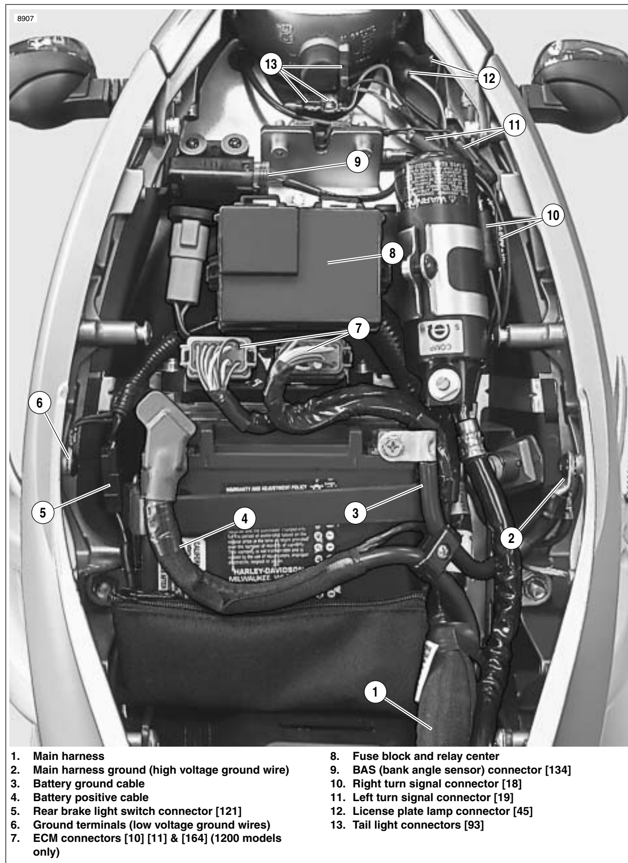
Figure 7-87. Main Harness and Electrical Connectors Under Seat
