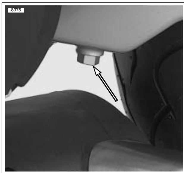
Figure 1-4. Oil Tank Drain Plug
