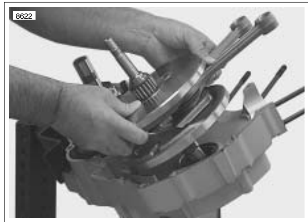
Figure 3-136. Removing Flywheels from Left Crankcase
