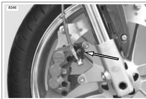
Figure 1-7. Front Caliper Bleeder Valve
