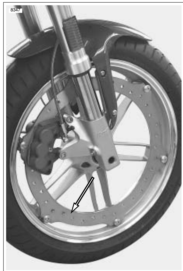
Figure 1-14. Front Brake Rotor
