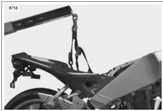
Figure 3-24. Supporting Vehicle for Disassembly
