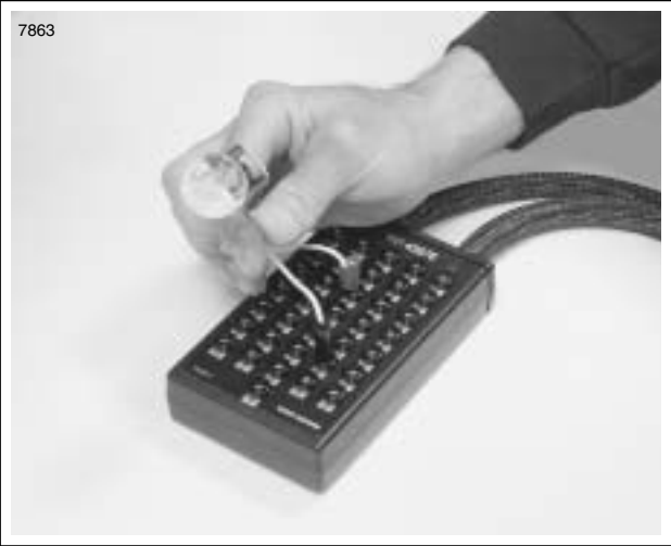
Figure 4-20. Ignition Coil Circuit Test
