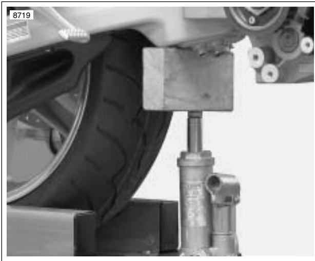
Figure 3-38. Supporting the Swingarm
