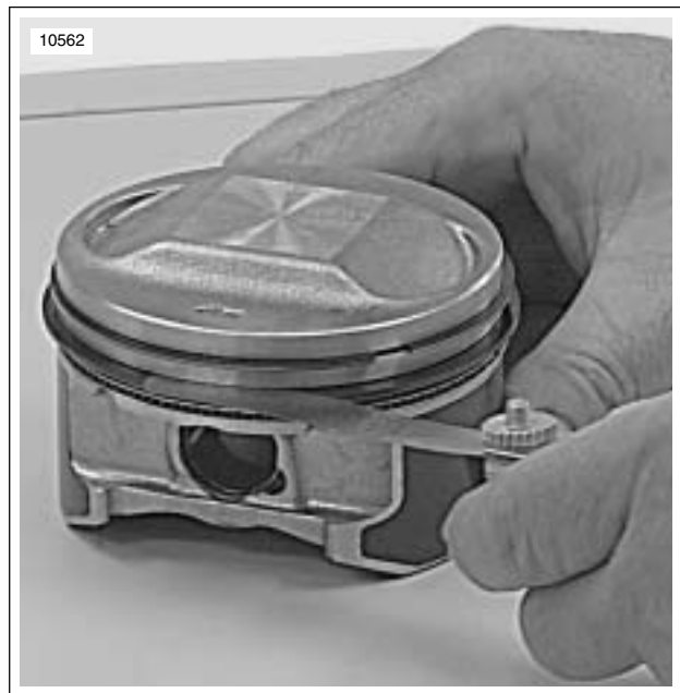
Figure 3-99. Measuring Ring Clearance in Groove
