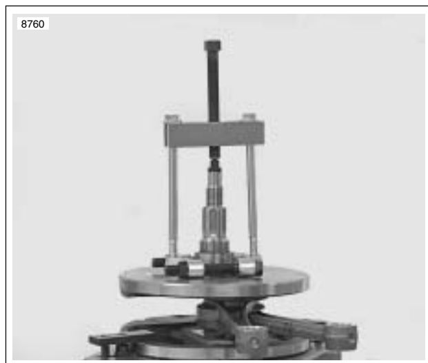
Figure 3-138. Removing Sprocket Shaft Inner Bearing Race
