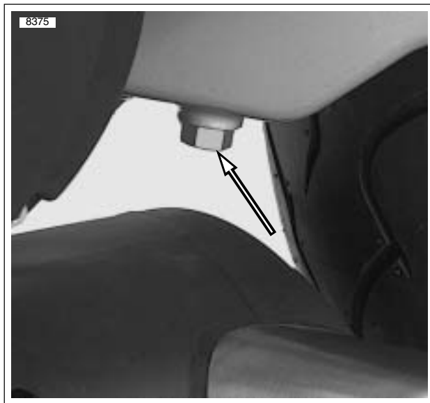
Figure 1-4. Oil Tank Drain Plug
