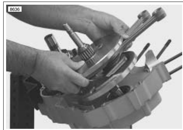
Figure 6-56. Removing Flywheels from Left Case Half
