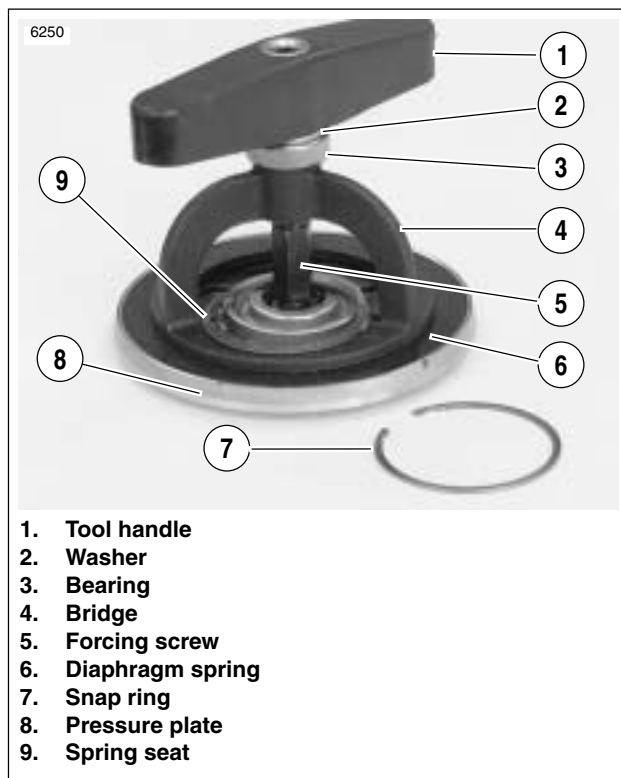
Figure 6-22. Pressure Plate Assembly
