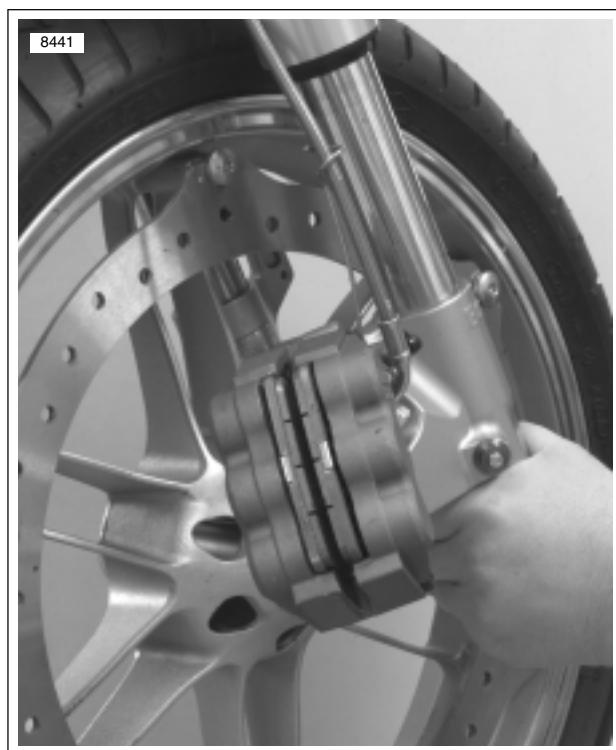
Figure 2-5. Front Wheel Removal
