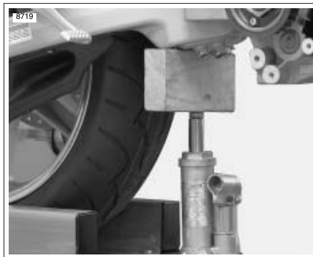
Figure 3-26. Supporting the Swingarm
