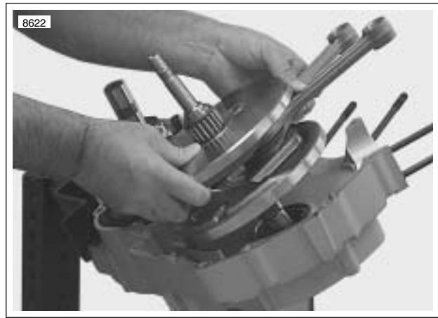
Figure 3-136. Removing Flywheels from Left Crankcase
