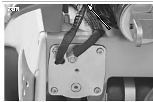
Figure 4-109. Fuel Pump connector [86] (swingarm removed for illustration)
