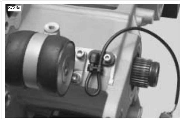
Figure 3-34. Rear Isolator and Mounting Hardware
