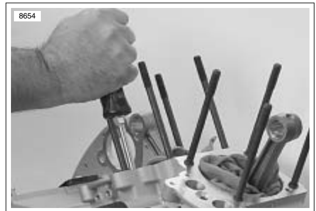
Figure 3-132. Checking Cam Gear End Play
