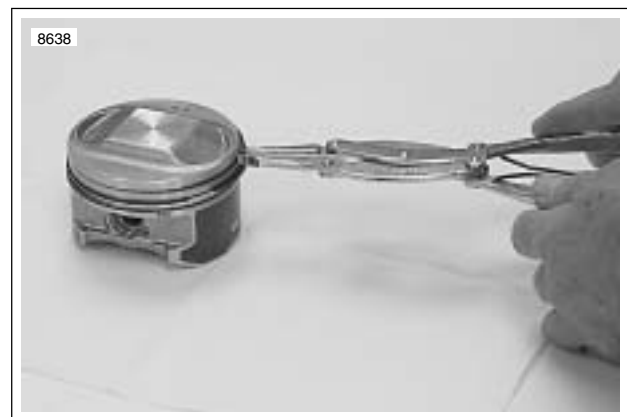
Figure 3-92. Removing Piston Rings
