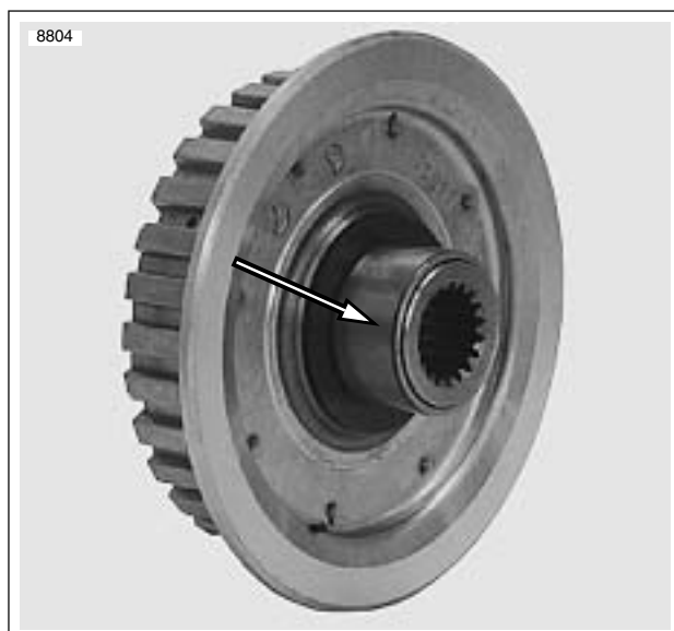
Figure 6-28. Clutch Hub Bearing Race
