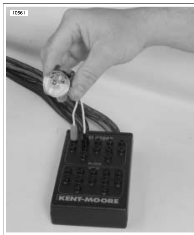
Figure 4-49. Testing Ignition Coil Connectors
