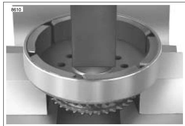
Figure 7-33. Removing Rotor From Sprocket
