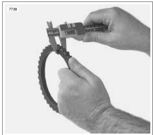
Figure 6-17. Measuring Friction Plates
