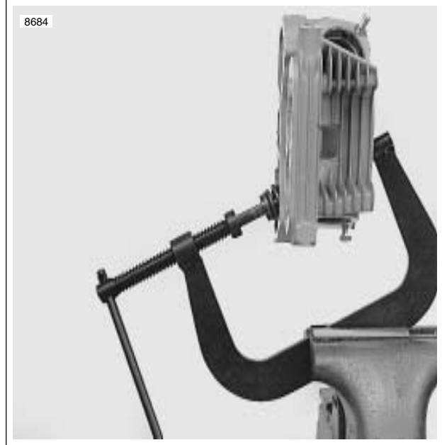
Figure 3-82. Valve Spring Compressor (Part No. HD-34736B)
