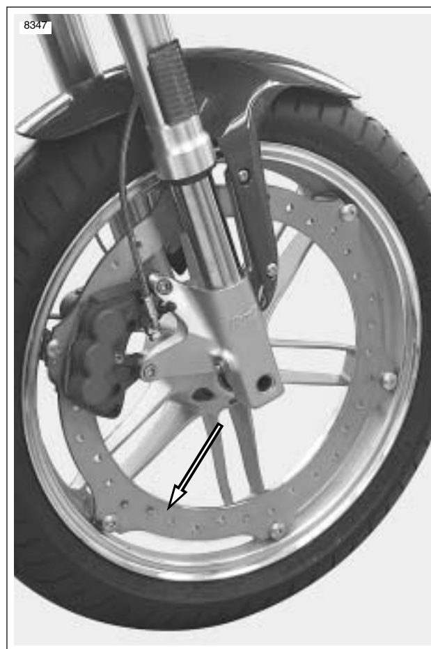
Figure 1-14. Front Brake Rotor
