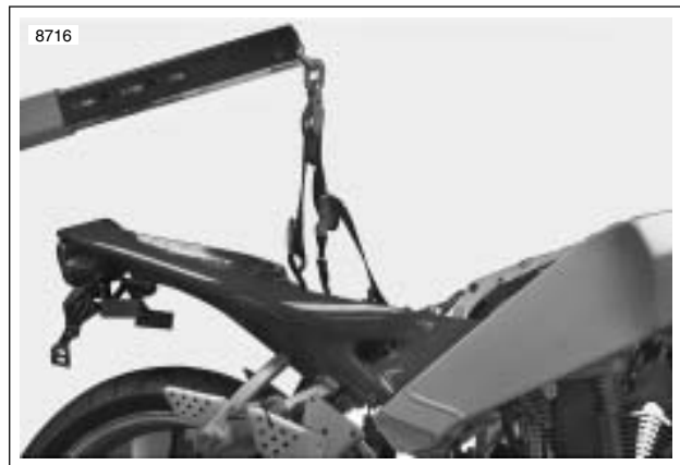
Figure 3-41. Supporting Vehicle for Assembly
