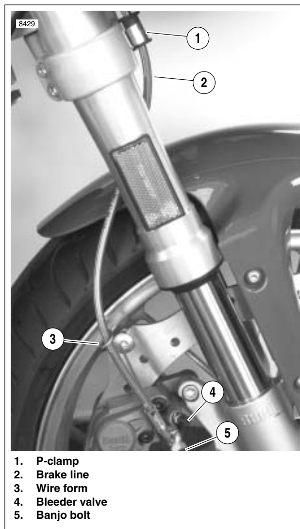
Figure 2-43. Front Brake Line
