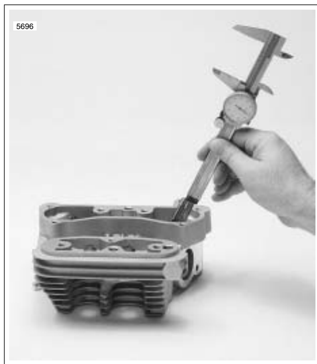
Figure 3-71. Measuring Valve Stem Protrusion
