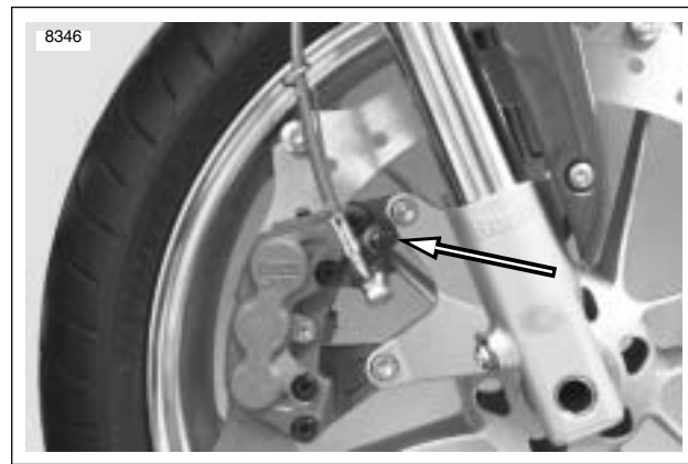
Figure 1-7. Front Caliper Bleeder Valve
