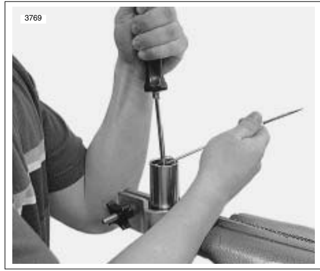
Figure 2-93. Compressing Spring Seat to Install Stopper Ring
