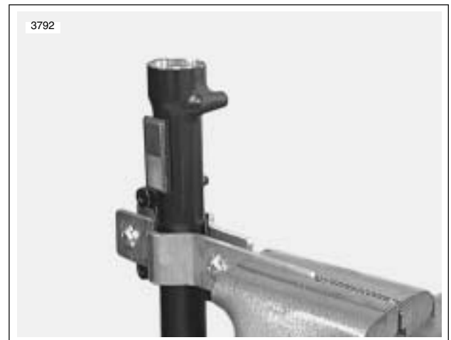
Figure 2-82. Clamping the Slider Assembly
