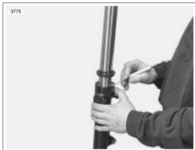
Figure 2-74. Removing Dust Seal
