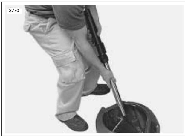
Figure 2-71. Pumping Fork Oil
