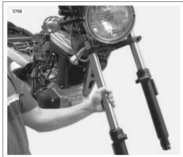
Figure 2-66. Front Fork Removal
