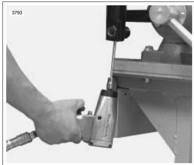
Figure 2-85. Install Center Bolt
