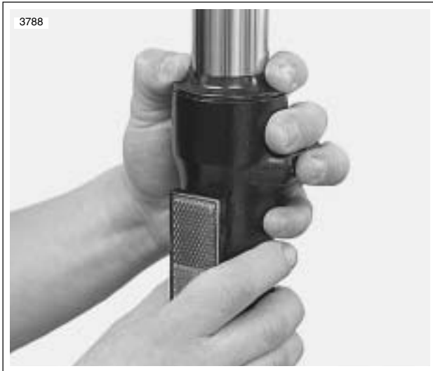
Figure 2-91. Install New Dust Seal
