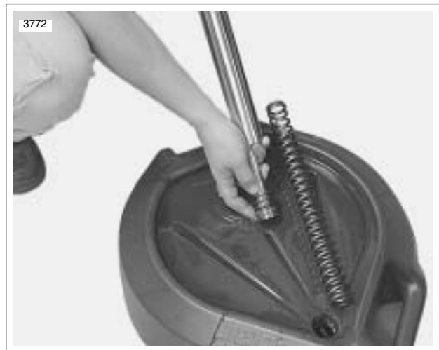
Figure 2-73. Removing Damper
