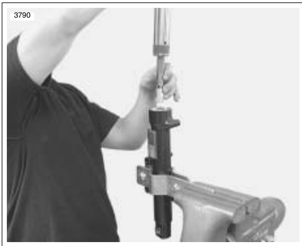
Figure 2-83. Installing Slider Tube
