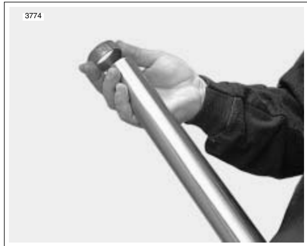
Figure 2-86. Install Guide Bushing
