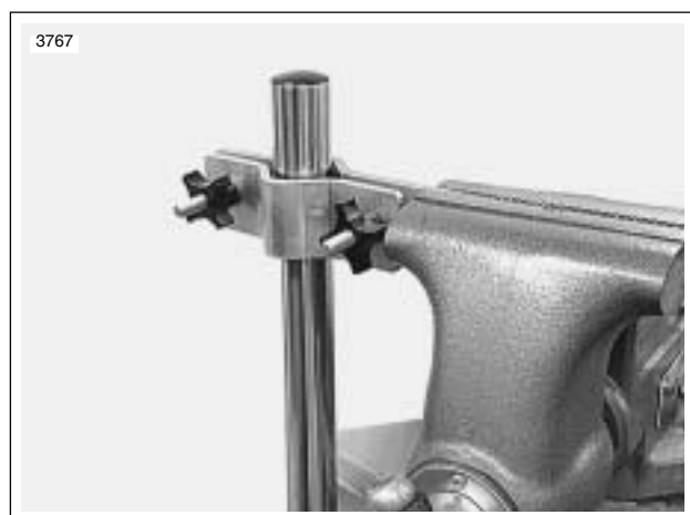
Figure 2-67. Clamping the Fork
