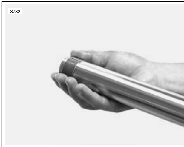
Figure 2-79. Install Slide Bushing
