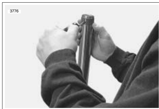
Figure 2-76. Removing Slide Bushing
