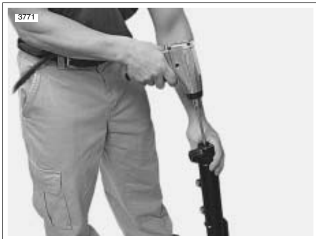
Figure 2-72. Removing Center Bolt
