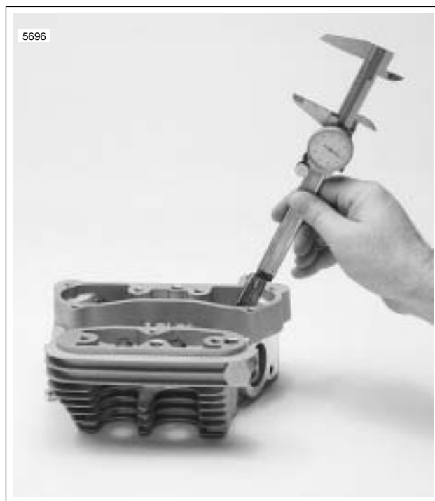
Figure 3-71. Measuring Valve Stem Protrusion
