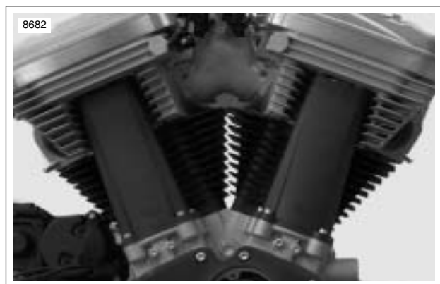
Figure 3-83. Push Rod Locations
