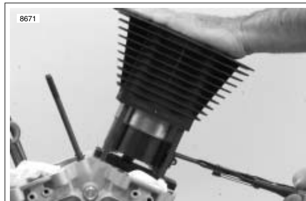
Figure 3-109. Compressing Piston Rings
