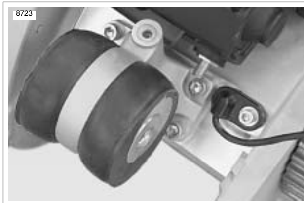
Figure 3-34. Rear Isolator and Mounting Hardware
