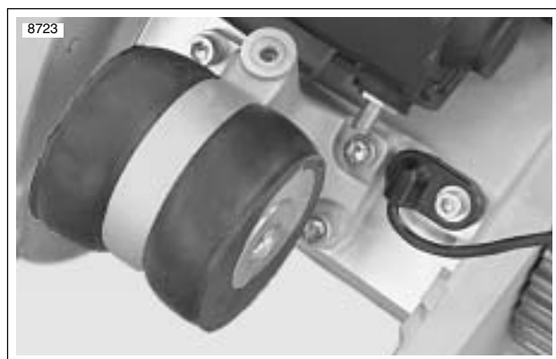
Figure 6-50. Rear Isolator Assembly
