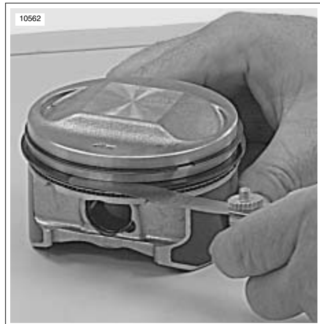
Figure 3-99. Measuring Ring Clearance in Groove
