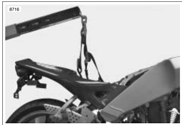
Figure 3-41. Supporting Vehicle for Assembly
