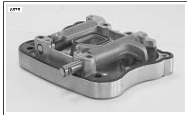
Figure 3-62. Removing Rocker Arm Shafts
