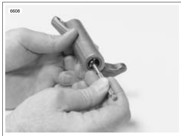
Figure 3-70. Measuring Rocker Arm Bushing Inner Diameter
