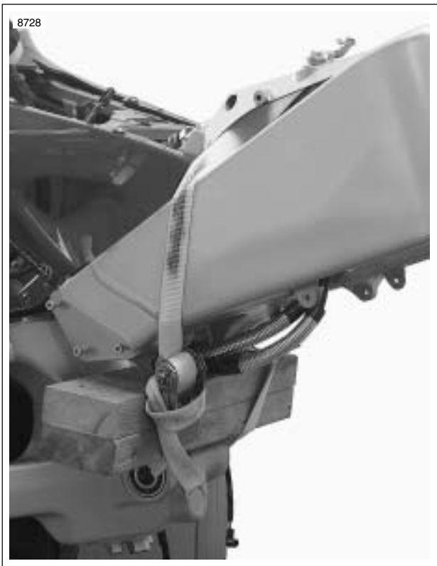
Figure 3-32. Securing Vehicle for Relocation
