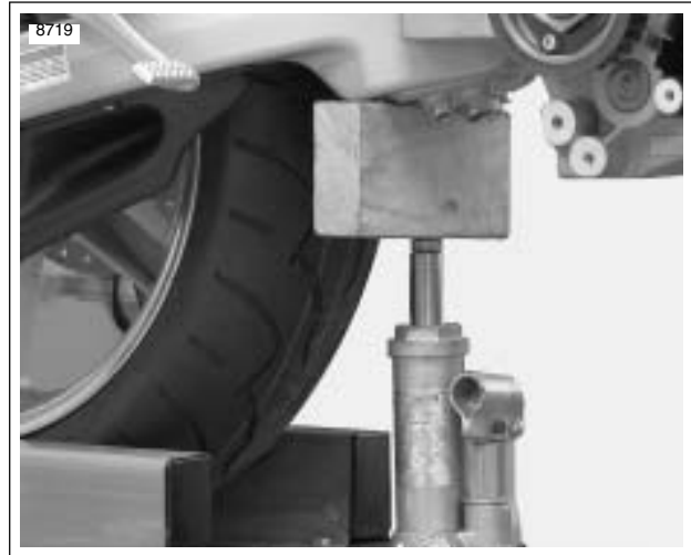
Figure 3-26. Supporting the Swingarm
