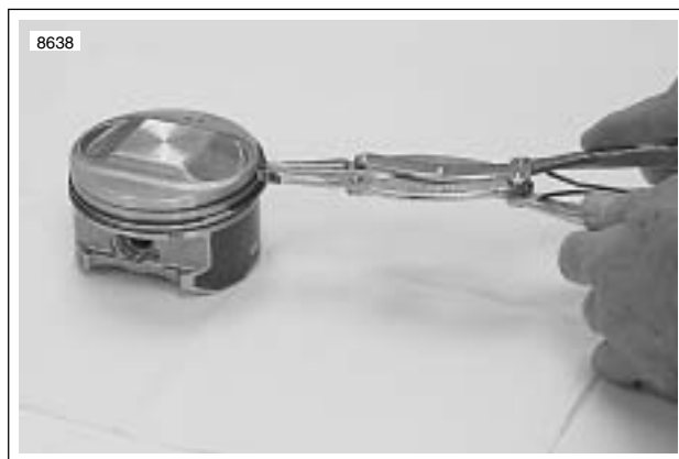
Figure 3-92. Removing Piston Rings
