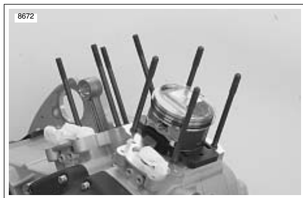
Figure 3-108. Piston Support Plate
