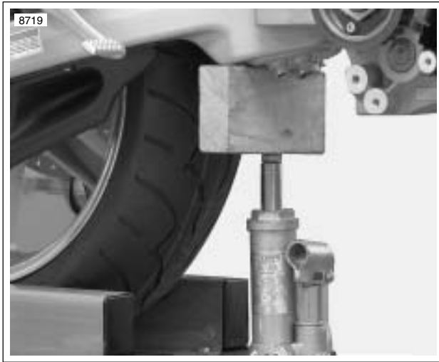
Figure 3-38. Supporting the Swingarm
