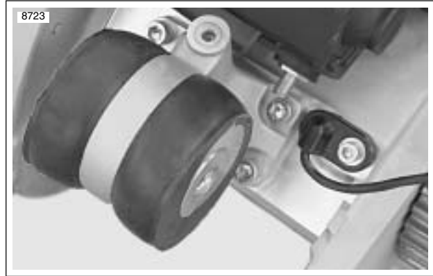
Figure 3-131. Rear Isolator Assembly
