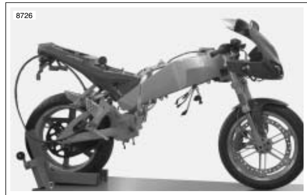
Figure 3-33. Rolling Chassis
