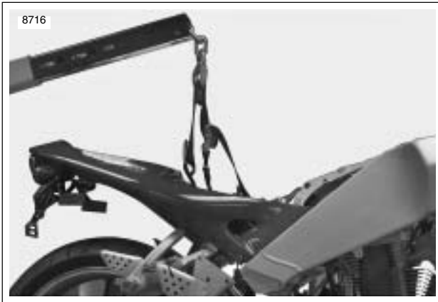
Figure 3-24. Supporting Vehicle for Disassembly
