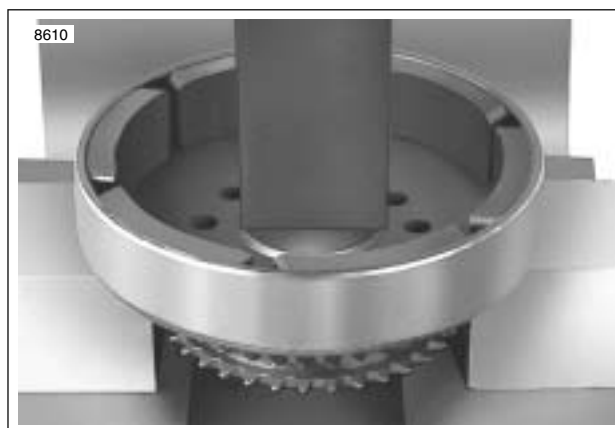
Figure 7-30. Removing Rotor From Sprocket
