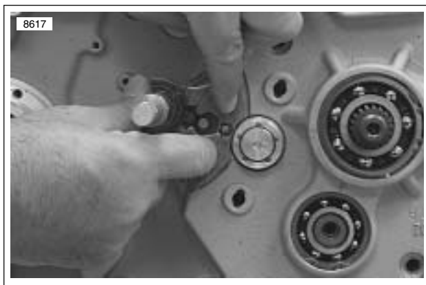
Figure 6-47. Removing Shifter Shaft Assembly
