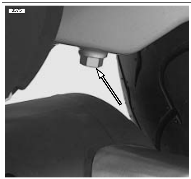
Figure 1-4. Oil Tank Drain Plug
