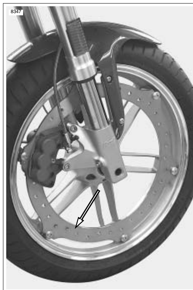
Figure 1-14. Front Brake Rotor
