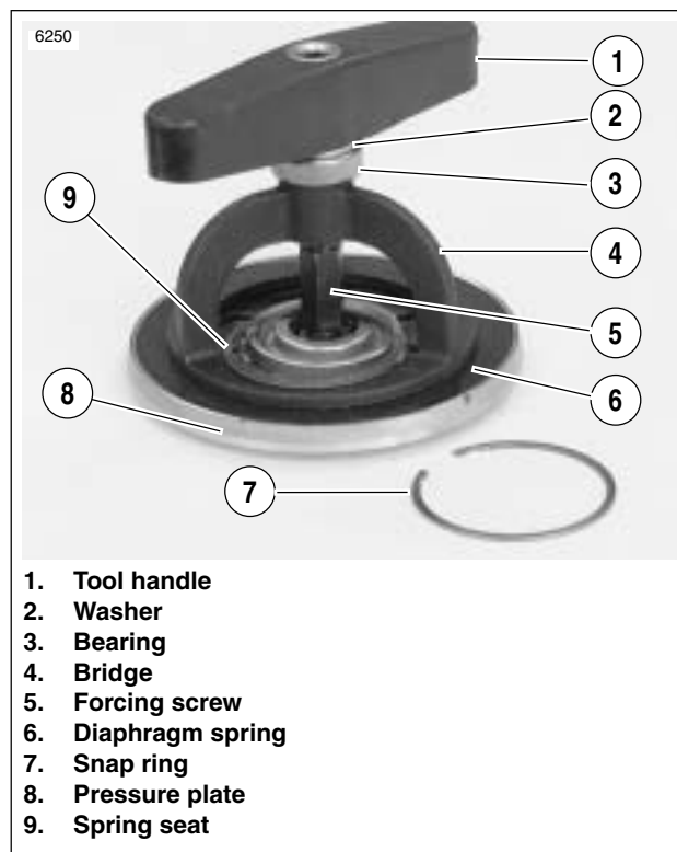
Figure 6-34. Pressure Plate Assembly
