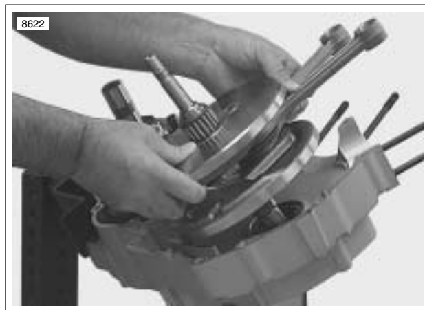
Figure 3-136. Removing Flywheels from Left Crankcase
