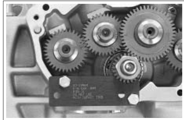
Figure 3-130. Crankshaft Locking Tool (Part No. HD-43984)
