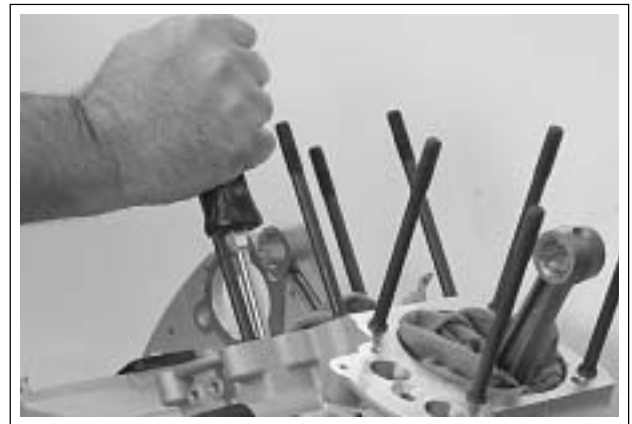
Figure 3-132. Checking Cam Gear End Play
