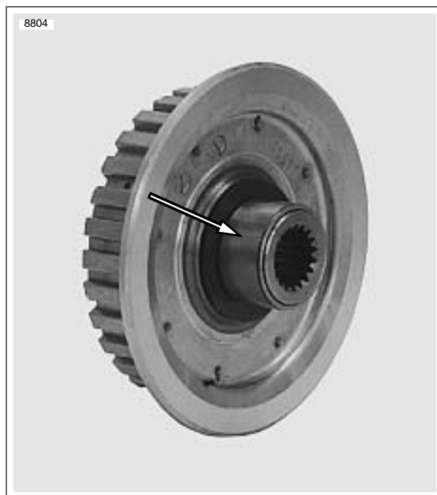
Figure 6-25. Clutch Hub Bearing Race
