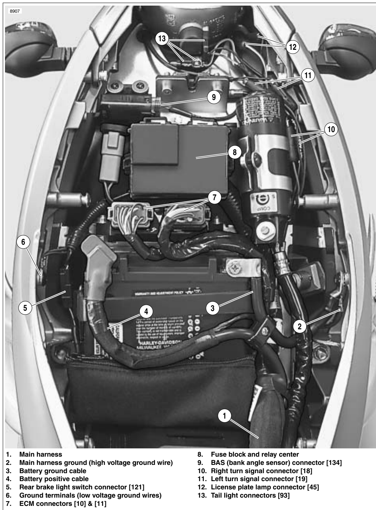
Figure 7-78. Main Harness and Electrical Connectors Under Seat
