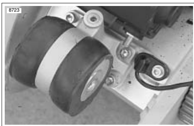
Figure 6-49. Rear Isolator Assembly
