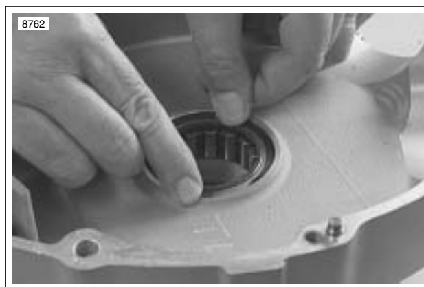
Figure 3-140. Removing Left Main Bearing Retaining Ring
