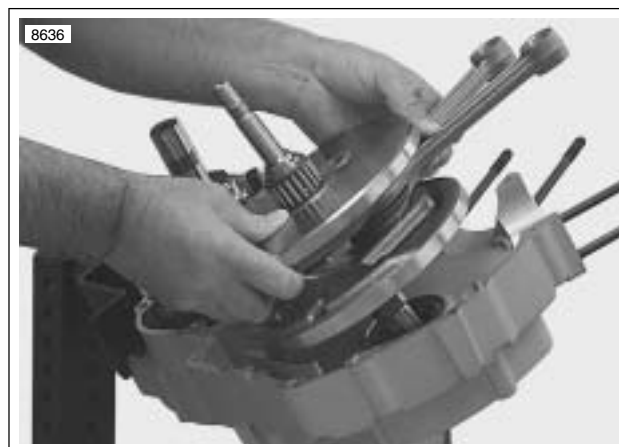
Figure 6-54. Removing Flywheels from Left Case Half
