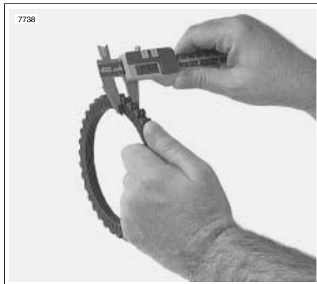
Figure 6-22. Measuring Friction Plates
