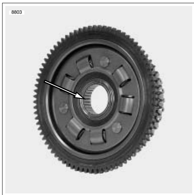
Figure 6-24. New Needle Bearing in Clutch Shell
