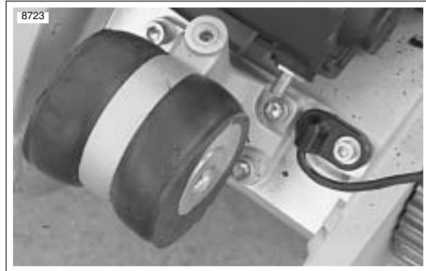
Figure 3-133. Rear Isolator Assembly
