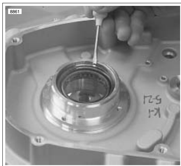
Figure 3-139. Left Main Seal Retaining Ring
