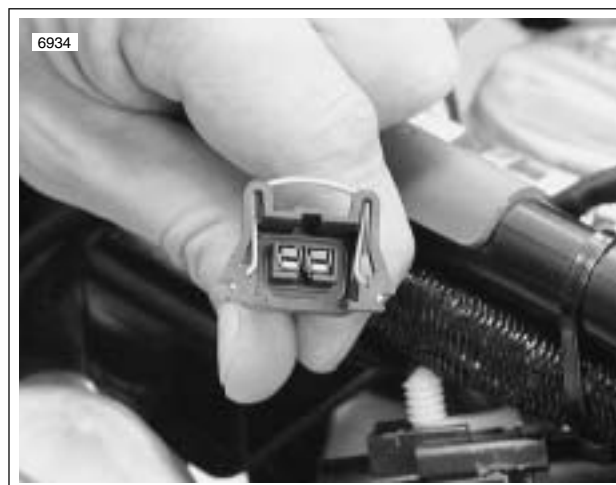
Figure 4-52. Fuel Injector Connector
