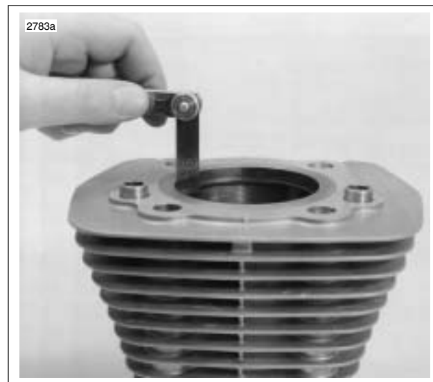
Figure 3-36. Measuring Ring End Gap
