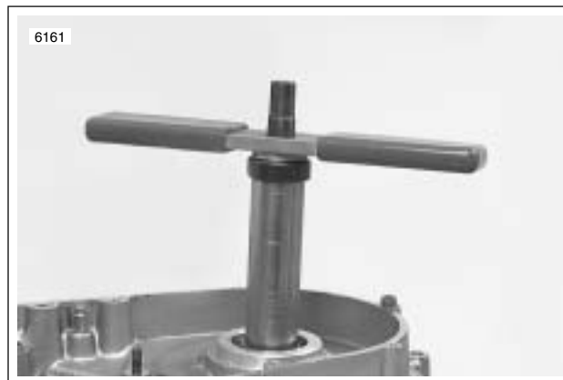
Figure 3-94. Installing Flywheel Spacer and Outer Bearing
