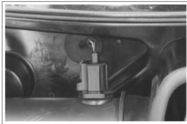
Figure 4-84. Intake Air Temperature Sensor Installed
