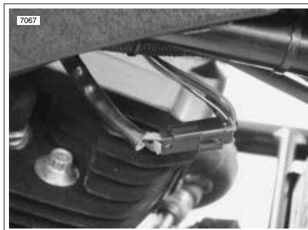
Figure 4-32. Fuel Pump Connector [86]
