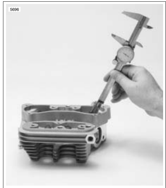
Figure 3-23. Measuring Valve Stem Protrusion
