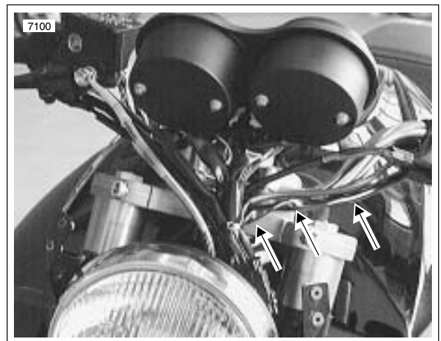
Figure 7-53. Routing Handlebar Wires, Left
