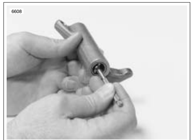
Figure 3-15. Measuring Rocker Arm Bushing Inner Diameter
