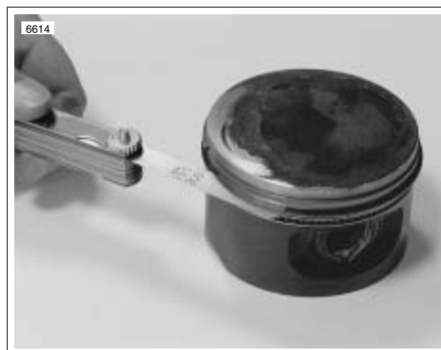
Figure 3-39. Measuring Ring Clearance in Groove
