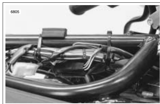
Figure 7-59. Speedometer Wiring Connector Locations (Approximate)
