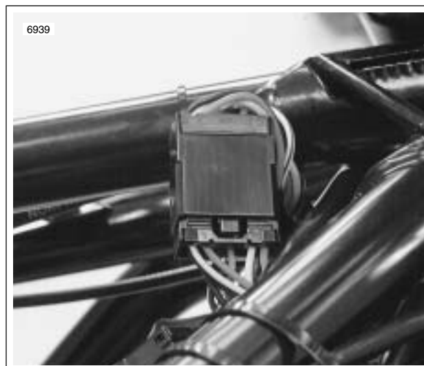
Figure 4-61. Speedometer/Tachometer Connector [39]
