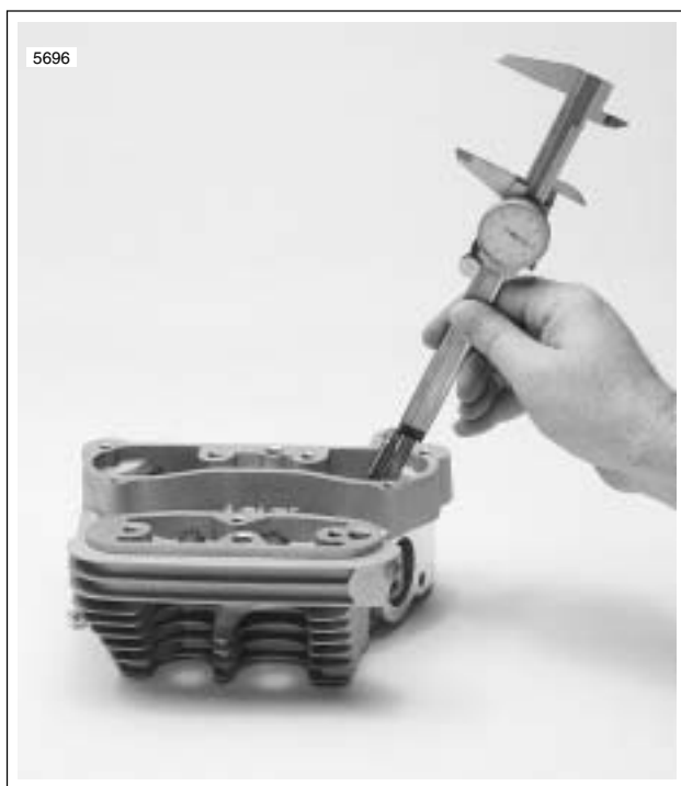
Figure 3-55. Measuring Valve Stem Protrusion
