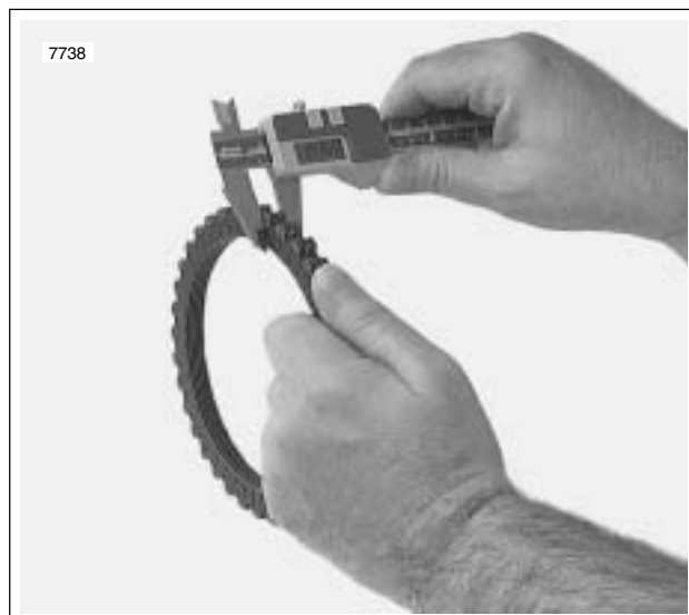
Figure 6-17. Measuring Friction Plates
