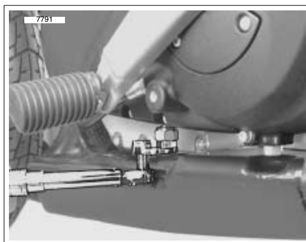
Figure 6-6. Torquing Chain Limiting Screw
