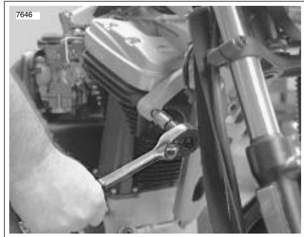
Figure 3-40. Cylinder Head Bolt
