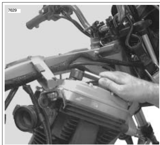
Figure 3-42. Install Crankcase Breather Hose
