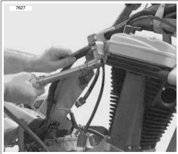
Figure 3-38. Install Top Rear Tie Bar
