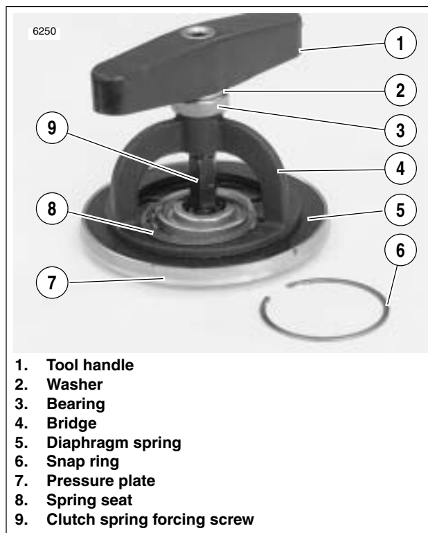
Figure 6-13. Pressure Plate Assembly
