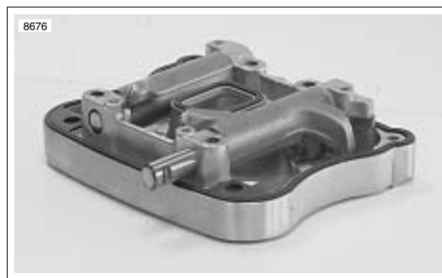
Figure 3-46. Removing Rocker Arm Shafts
