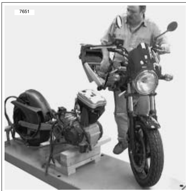
Figure 3-26. Move Chassis to Engine
