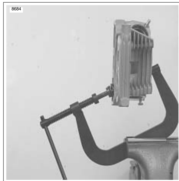
Figure 3-48. Valve Spring Compressor (Part No. HD-34736B)
