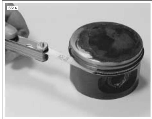
Figure 3-79. Measuring Ring Clearance in Groove
