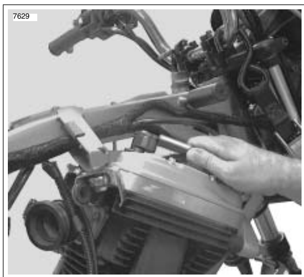
Figure 3-1. Remove Crankcase Breather Hose
