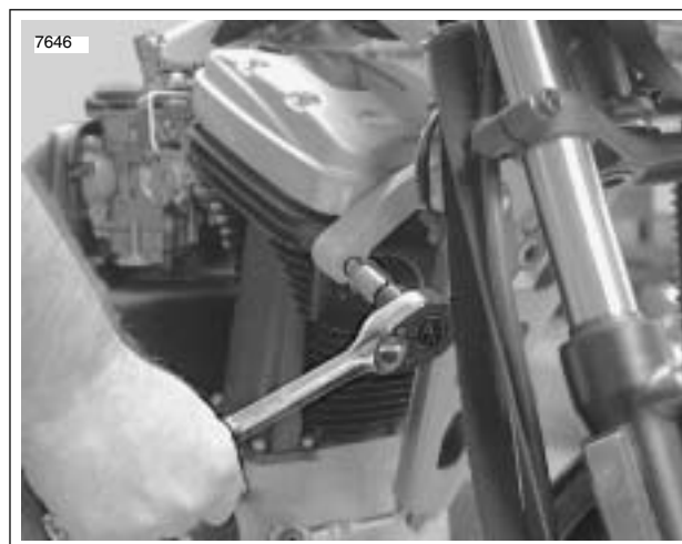
Figure 3-2. Cylinder Head Bolts
