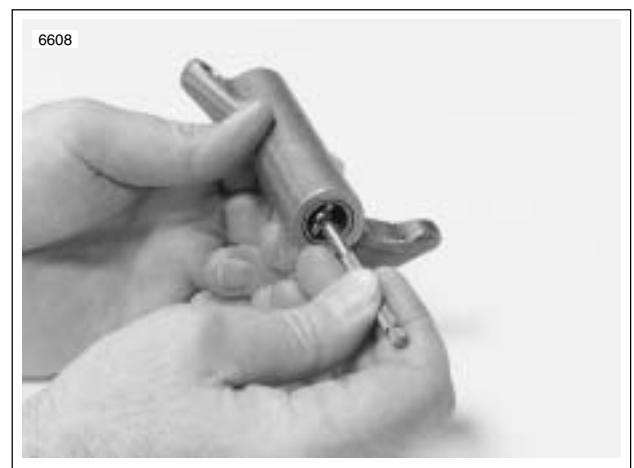
Figure 3-54. Measuring Rocker Arm Bushing Inner Diameter
