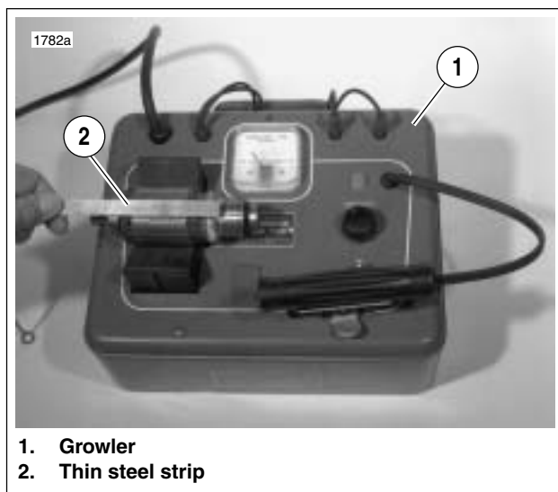
Figure 5-20. Shorted Armature Test Using Growler
