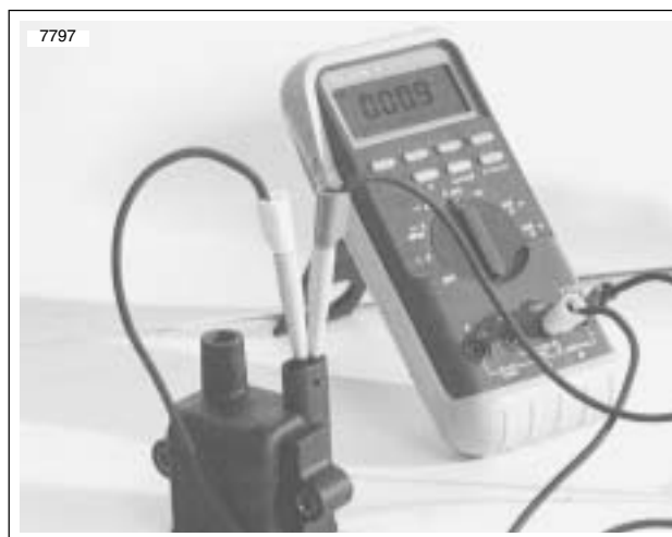
Figure 7-25. Ignition Coil Primary Resistance Test
