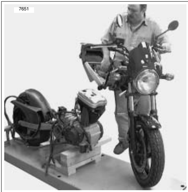
Figure 3-15. Move Chassis From Engine
