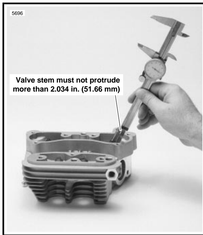
Figure 3-22. Measuring Valve Stem Protrusion
