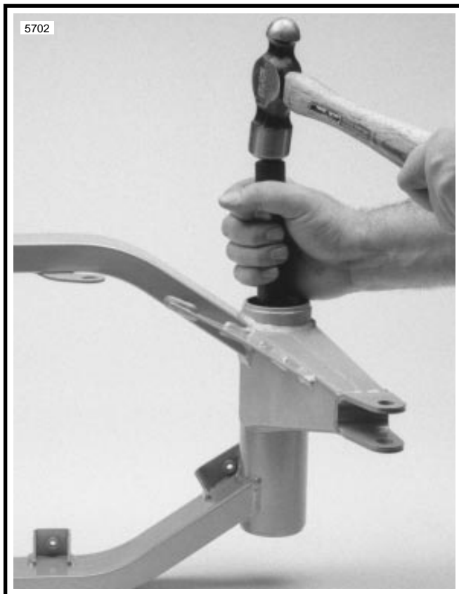
Figure 2-38. Removing Roller Bearing Cups
