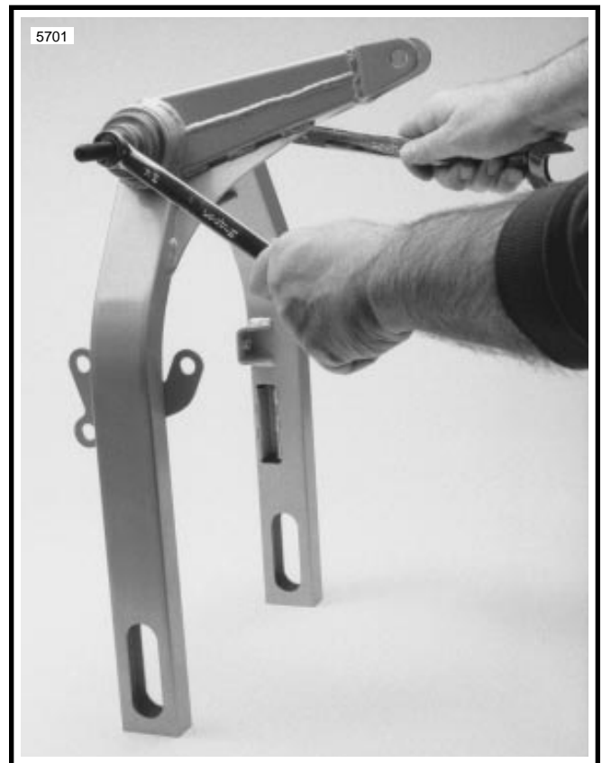
Figure 2-39. Installing Bearings into Swingarm
